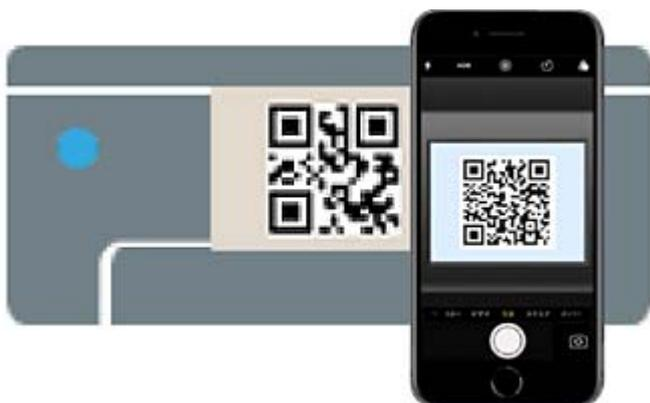
Use the Camera app for iOS 11 or later. You cannot connect to the printer using the Camera app for iOS 10 or earlier. Also, you cannot connect using an app for scanning QR codes. If you cannot connect, select **Other Methods** on the printer's control panel. See the related information link below for details on connecting.
