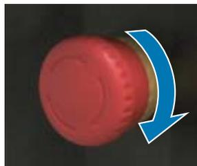
To release the emergency stop, turn the button clockwise. Next, press the power on ( | ) button to return the printer to normal status.
