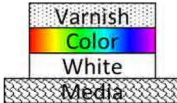
When set to [Forward], the gantry prints while moving from back to front. When all of the white, color, and varnish layers have been printed, the printing status is as shown below.
