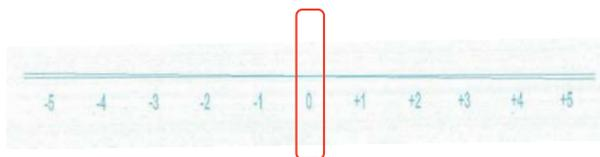
For example, if the "0" line is not straight but the "+1" line is straight, add "+1" to the original value shown on the screen and enter it. When you have finished entering the numbers, press [Register].
