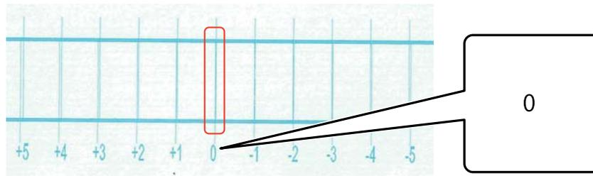
If the "0" line is not straight but the "+1" line is straight, for example, add "+1" to the original number on the screen, and then enter it.
