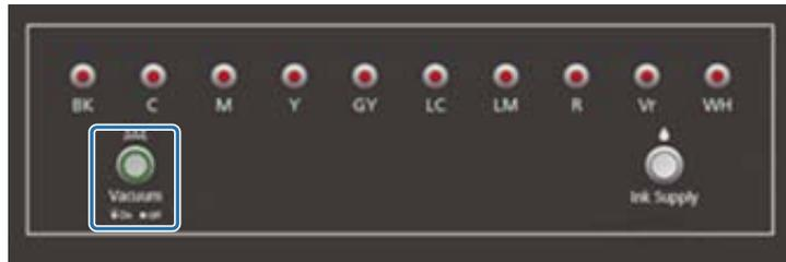
2-2 Open the valve according to the position in which the media is loaded. The media sticks to the table.
