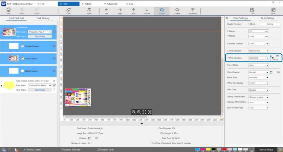
When set to [Backward], the gantry prints while moving from front to back. When all of the white, color, and varnish layers have been printed, the printing status is as shown below.
