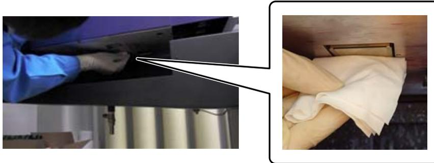
Wipe the surface of the nozzles from back to front. Do not wipe in the opposite direction.
