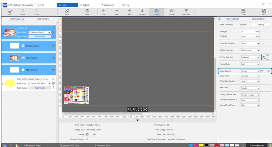
You can use [Color Channel] to specify the layer you want to print. Select from [Normal], [Only Color], [Only White], [Only Varnish], [Color and White], [Color and Varnish], and [White and Varnish] according to your printing needs. If you select [Normal], layers are printed according to the data sent.
