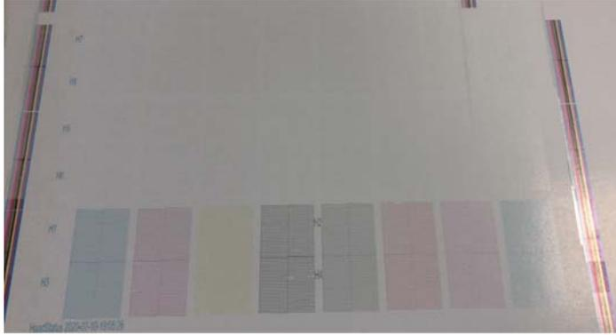
The white ink is white and varnish is transparent with patterns printed on them. Check these by using reflected light.
