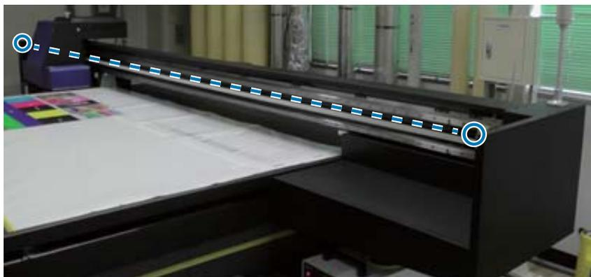
If someone enters the operating range of the carriage, this sensor detects the movement and immediately stops the carriage. Sensors are attached at the positions shown in the photo.
