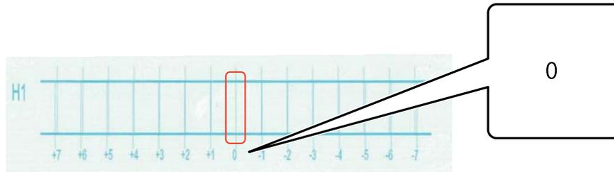
If the "0" line is not straight but the "+1" line is straight, for example, add "+1" to the original number on the screen, and then enter it. When you have finished checking the pattern for each print head (H1 to H8) and entering the values on the screen, press [Register].
