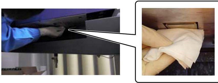
Wipe the surface of the nozzles from back to front. Do not wipe in the opposite direction.
