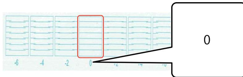
If the "0" line is not straight but the "+1" line is straight, for example, add "+1" to the original number on the screen, and then enter it. When you have finished checking the pattern for each print head (H1 to H8) and entering the values on the screen, press [Register].
