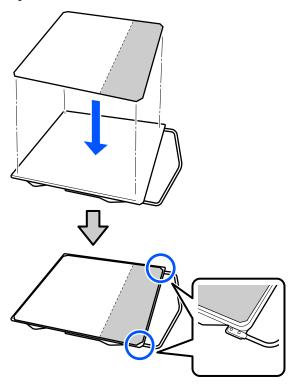
Gently press on the section from which the back has been peeled off the grip pad to stick the grip pad onto the platen.
