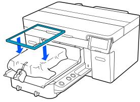
Remove any lint from the printing surface, and press the fibers flat.
