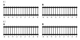
Check the two patterns A to B in each block, and select from -8 to +8, where the line appears thinnest (lines overlap) in the pattern.
