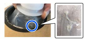
This is a result of coagulation of the fixing component in the pre-treatment liquid. If you use the pre-treatment liquid with coagulation as it is, the print results will be uneven. Therefore, you need to filter it to remove the coagulation before use.
