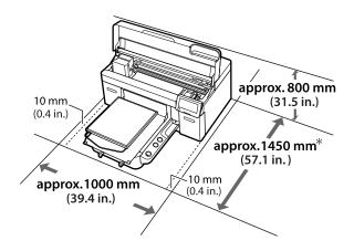
\*Approximately 1500 mm (59.1 in.) when the optional L size hanger platen is installed.
