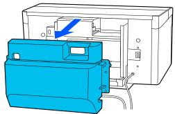
Remove the waste ink tubes by gripping them from below with a clean-room wiper as shown in the illustration, and then use it to wipe off the waste ink from the waste ink outlet.
