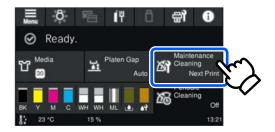
Operation areas do operations when pressed. As shown below, when a scroll bar is displayed, you can scroll the screen by moving (sliding) your finger up and down on the screen. You can also scroll by pressing on the up and down icons on the scroll bar.
