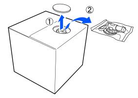
Pull the cap section out of the hole in the cardboard.
