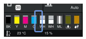
The dividing line between C and WH indicates which ink color is loaded inside the left or right ink cover when viewed from the front of the printer.
