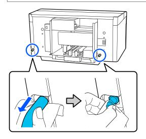
Attach the caps that you removed during setup to the waste ink outlets.
