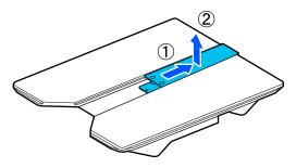
You need the removed screw and parts when loading polo shirts and so on. Store them in a safe place. We recommend keeping the screw attached to the platen.
