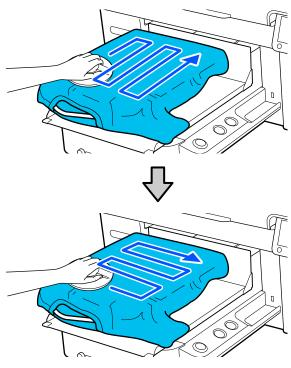
When loading a T-shirt coated with pre-treatment liquid, or when the grip pad tool gets caught due to the characteristics of the fabric, use the grip pad tool with a release sheet such as silicon paper on the T-shirt as shown in the figure.
