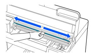
Wipe off ink stains by moving a clean-room wiper from the center of the encoder scale to either end of the scale, moving it back and forth about two or three times.
