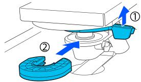
Loosen the fixing lever while lifting the ① part shown in the illustration.
