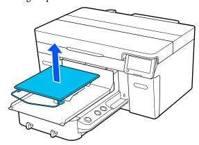
Make sure the protruding shaft of the replacement platen fit into the holes.
