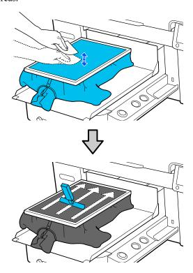
Pull the T-shirt outside of the frame to remove any creases and slack.
