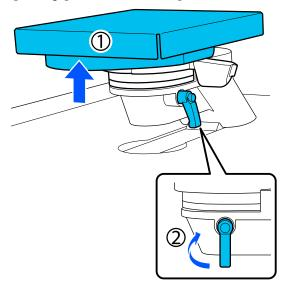
Lift the platen gap lever and remove the spacer.
