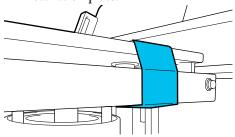
☐ Make sure the end of the fixing band is on the side of the platen.
