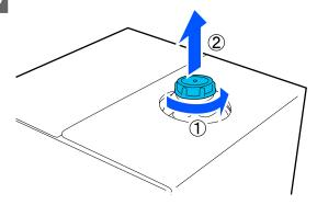
Remove the tap from the bag and check that the hole is visible.
