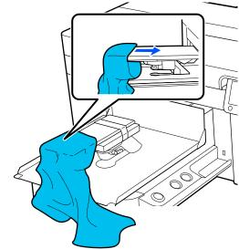
Pull the parts of the shirt that extend beyond the platen to flatten the print surface.
