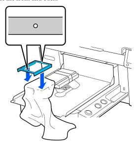
Pull the T-shirt outside of the frame to remove any creases and slack.
