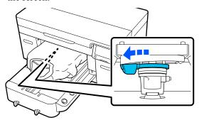
Move the lever one notch to the right to locate the position where the error sound stops.
