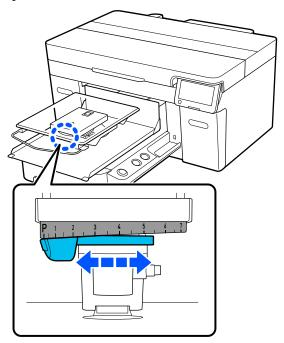
When the scale is at P, the platen is at its highest; the higher the number, the lower the platen.
