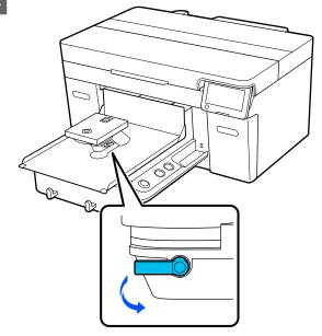
Move the platen gap lever to the right to set the scale to 8.
