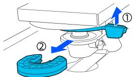
Combine spacers according to the type of platen being used and the thickness of the media.
