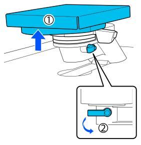
Release the part that was lifted in the previous step, and then tighten the fixing lever again to secure the platen gap lever.
