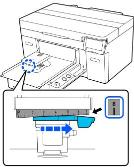
Tighten the fixing lever while lifting the ① part shown in the illustration, to secure the platen gap lever in the raised position.
