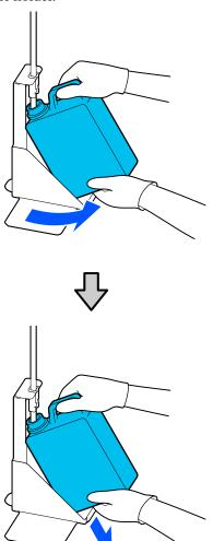
Insert the waste ink tube into the mouth of the new Waste Ink Bottle and place the Waste Ink Bottle in the holder.
