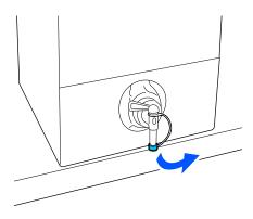
Open the lever to pour one liter of the pre-treatment liquid into the bottle through the filter.
