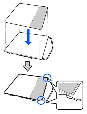
Gently press on the section from which the back has been peeled off the grip pad to stick the grip pad onto the platen.
