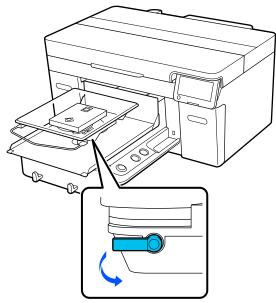
Move the lever clockwise to set the scale to P.
