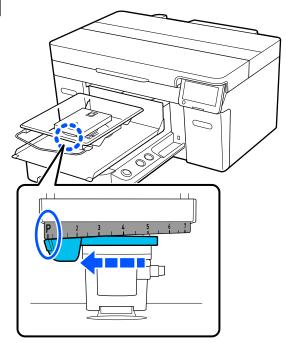
When the scale is at P, the platen is at its highest position; the platen position lowers as the number increases.
