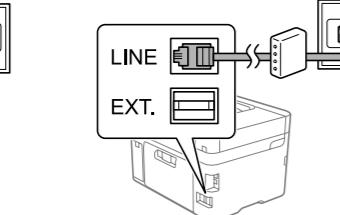
RJ-11 Phone Line / RJ-11 Telephone set connection
