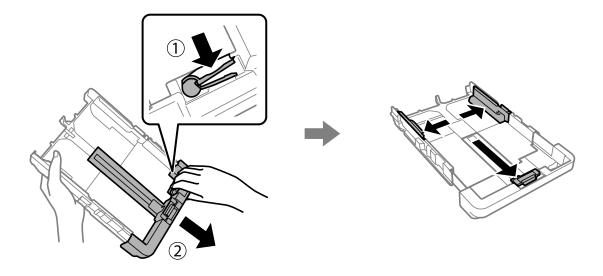
With the printable side facing down, load a single sheet of paper that does not extend beyond the triangle symbol at the end of the cassette. Slide the edge guide to the edge of the paper.
