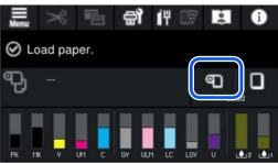
Press **How To...** to view the loading procedure. Follow the on-screen instructions to continue.
