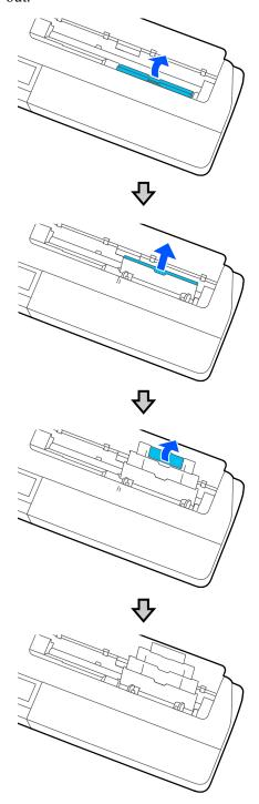
Load paper in the auto sheet feeder with the printable side facing you.
