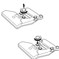
5. Remove the rectangular cap and attach it to the rectangular opening, as shown in the illustration below.
