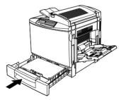
When the paper jam is cleared completely, the jammed page's print data is automatically reprinted.
