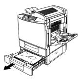
4. Gently remove any paper that has fed part way into the printer.
