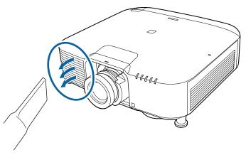
Loosen the screws and remove the air filter cover as shown (it is attached with a tether).
