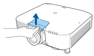
4. Remove the stopper, if necessary.
