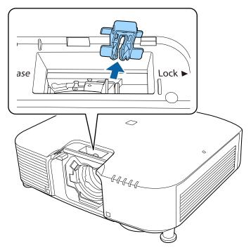
Pinch the lock lever and move it to the **Release** position.
