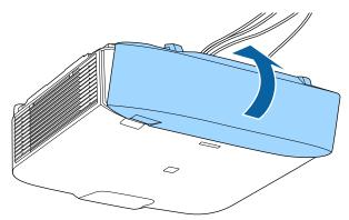
Tighten the cable cover screws.
