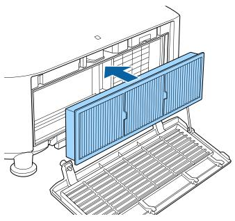
**5** Replace the air filter cover as shown and tighten the screws.
