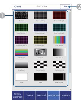
Displays available test patterns; select to project a test pattern.
