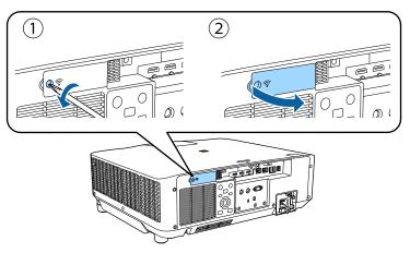
**3** Connect the Wireless LAN module to the wireless LAN module slot.
