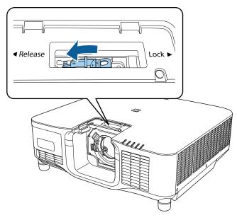
Insert the lens straight into the projector's lens socket with the white dot facing up.
