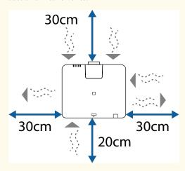
See the projector's *Specifications* for detailed locations of the air intake vent and air exhaust vent.
