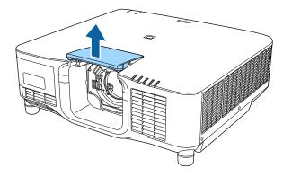
**3** Pinch the lock lever and move it to the **Release** position.
