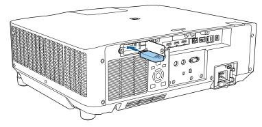
Replace the wireless LAN module cover as shown and tighten the screws.
