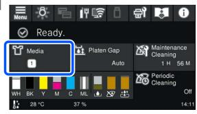
Press in the order of **Print Adjustments** - **Print Head Alignment**, and then select either **Standard** or **Micro Adjust**.
