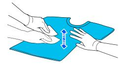
Squeeze the pre-treatment liquid out of the roller by pressing it against the edge of the tray, and apply the liquid evenly.
