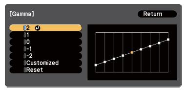
When you select a smaller value, you can reduce the overall brightness of the image to make the image sharper. When you select a larger value, the
