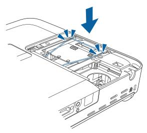
**9** Replace the lamp cover and tighten the screw to secure it.
