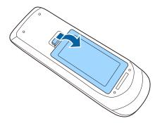
Insert the batteries with the + and - ends facing as shown.
