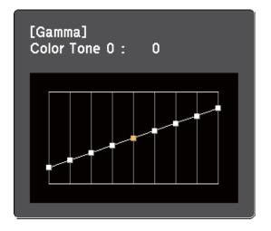
• To use the gamma adjustment graph, select **Adjust it from the graph**. Press the left or right arrow buttons to select the color tone you want to adjust. Then press the up or down arrow button to adjust the value and press [Enter].
