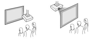
Make sure you select the correct **Projection** option in the projector's **Extended** menu according to the installation method being used.
