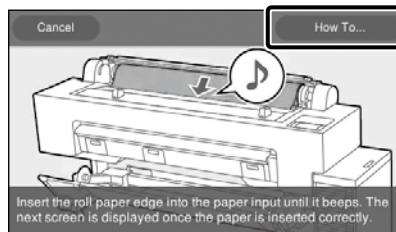
Example: When **Roll Paper** is selected Press **How to...** to display the setting procedure. After that, you can carry out the task while checking the procedure on the screen.
