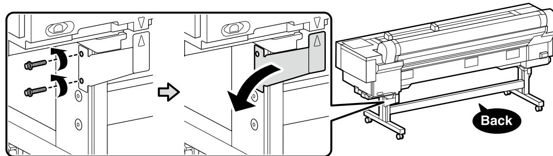
Removed parts will be used when reassembling the printer. Keep them in a safe place.
