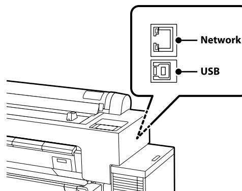
The computer must be connected to the Internet so that software can be downloaded during the installation. Ready the printer and computer for connection before proceeding, but do not connect the cables until the installer prompts you to do so. The basic software will not be installed if the devices are not connected according to the on-screen instructions.
