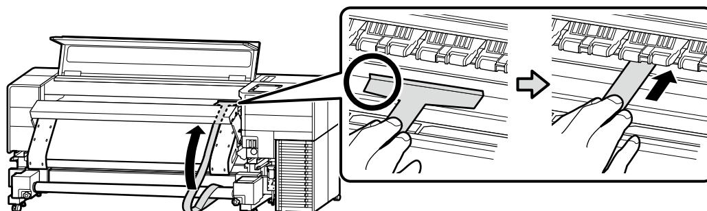
Turn around to the back side, and pull out the adjustment film ③ until it is stretched taut.
