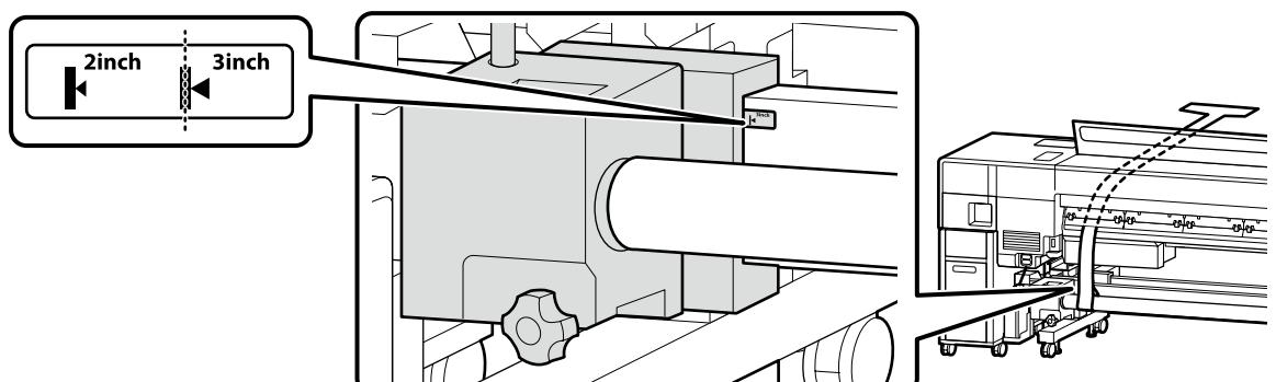
For step [7], set the adjustment film so that it is perpendicular to the paper tube.
