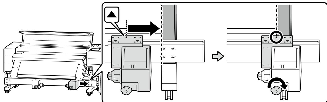
Move the media holder on the side opposite the control panel to the edge, and turn the handle until it no longer turns.
