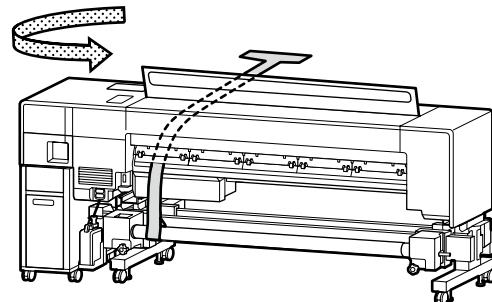
On the back side, for step [4], align the edge of the media holder with the 3-inch mark.
