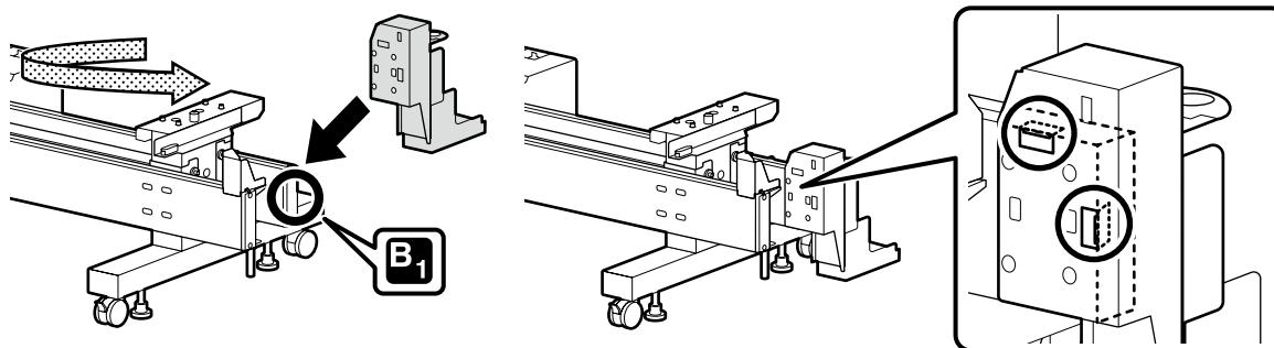
Install the component so that both two parts circled by ○ touch the edge of the stand.
