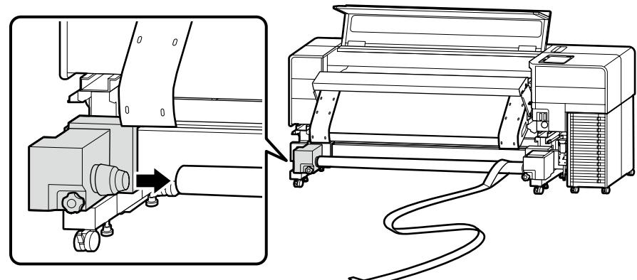
Hold the groove on the side of the media holder with both hands, and push the media holder into paper tube ② twice before locking the locking lever.
