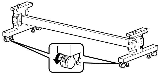
Before using the printer, be sure the stand is fixed in place. When moving the printer, unlock the casters.
