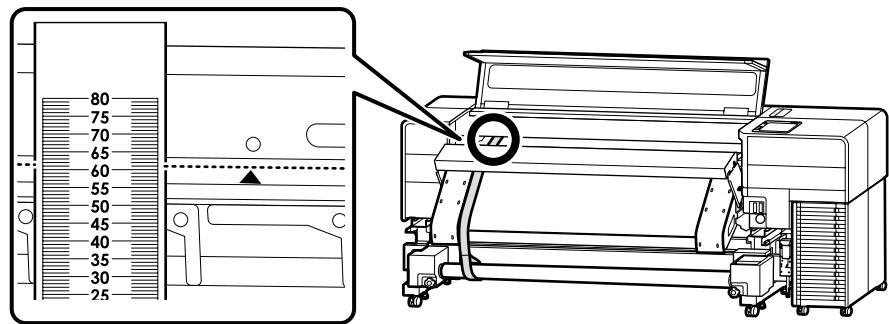
Similarly on the side opposite the control panel, record the value at which the edge indicated by the ▲ mark on the printer overlaps the scale on the adjustment film.
