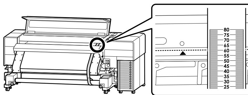
Record the value at which the edge indicated by the ▲ mark on the printer overlaps the scale on the adjustment film.
