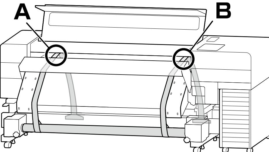
Perform parallel adjustment to align the length of the print path on the left and right (A and B in the figure).
