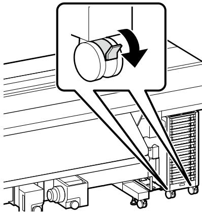
Before using the printer, be sure the stand is fixed in place. When moving the printer, unlock the casters.
