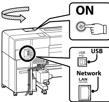
Before starting the installation, enable the connection between this printer and the computer. Connect the computer to the Internet to download and install the software. Connection between this printer and the computer via a cable must be done by following the on-screen instructions during installation. Doing so in advance will not allow the basic software to be installed.
