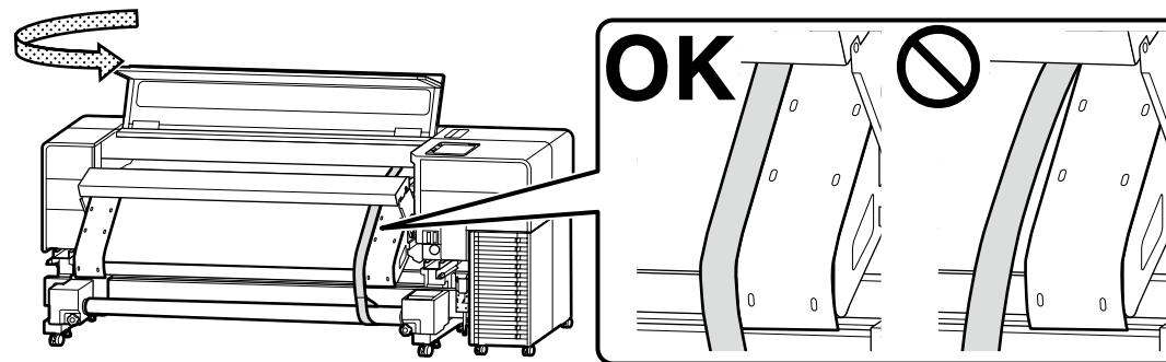
Be sure to align the adjustment film with the guide.
