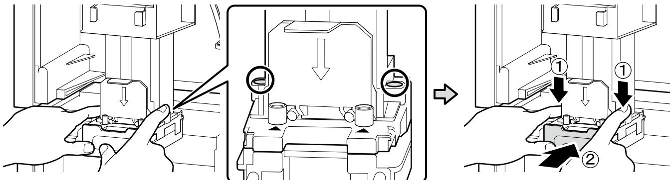
To securely connect the ink path, lock the lever while firmly pressing the parts circled by O from above with both hands.
