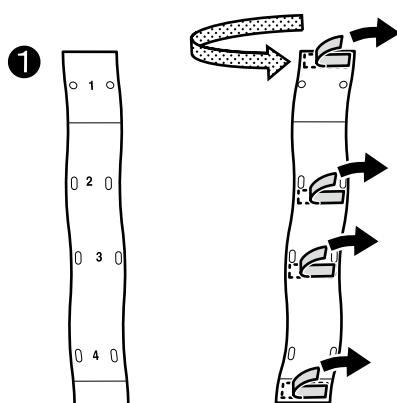
Attach guides ① to both the left and right sides in order to fit holes 1-4 with the screws at the end of the heater.
