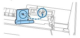
Tighten the screw with a cross-head screwdriver to secure the cutter.
