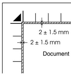
An area  $2 \pm 1.5$  mm in from both horizontal and vertical rulers will not be scanned.
