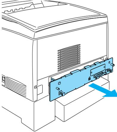
4. Identify the memory slot. Its position is shown below.
