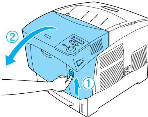
2. Grasp the two orange tabs and pull the unit forward and down, then lift the unit out of the printer.
