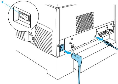
2. Remove all interface cables from the interface connectors.
