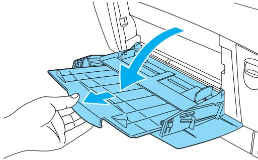
2. Load a stack of the desired media with the printable surface facing down, then slide the guides against the sides of the stack to get a snug fit.
