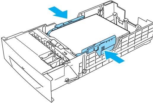
6. Insert the paper cassette gently into the printer, and push it back into the printer.
