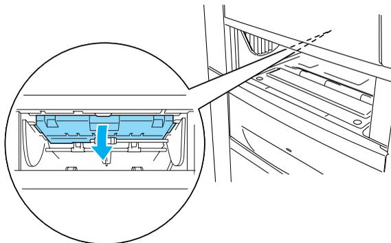
When the paper jam is cleared completely and cover A is closed, printing resumes from the page that jammed.
