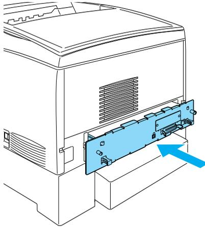
8. Fasten the circuit board tray with the two screws.
