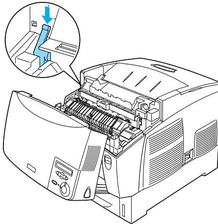
4. Unlock the locks on both sides of the fuser unit.
