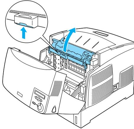
4. Hold the photoconductor unit by the handle, and slowly lift it straight out of the printer.
