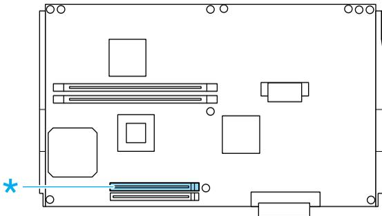
6. Push down on the tab on the right side of the ROM slot to raise the module out of the slot A.
