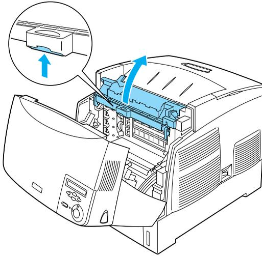
4. Grasp the handle of the photoconductor unit firmly and remove the unit from the printer.
