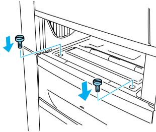
9. Remove the cover on the back of the standard lower cassette, and secure the back of the unit to the printer with the remaining two screws. Then reattach the cover.
