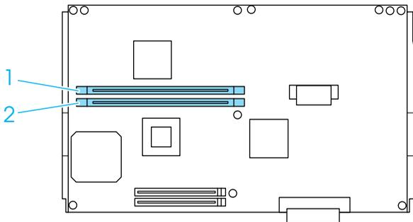
6. Grasp both sides of the memory module and pull the module out.
