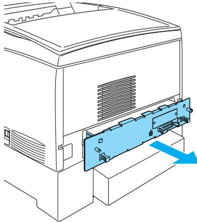
5. Identify the memory slot. Its position is shown below.
