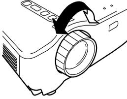
1. Turn the focus ring on the projector to adjust the focus.
