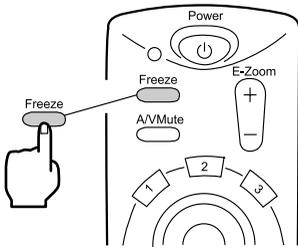
1. Press the Freeze button on the remote control.
