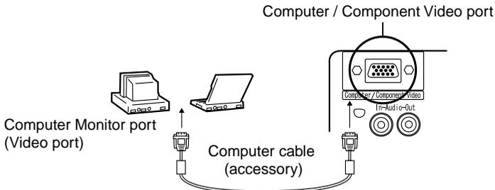
\* If your computer port style is not a mini D-Sub 15-pin interface, use a connection adapter that provides this interface.
