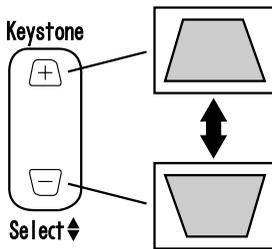
1. Press the Keystone button on the projector to minimize the trapezoidal distortion.
