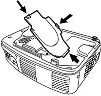
2. After the projector has cooled completely, remove the lamp cover.
