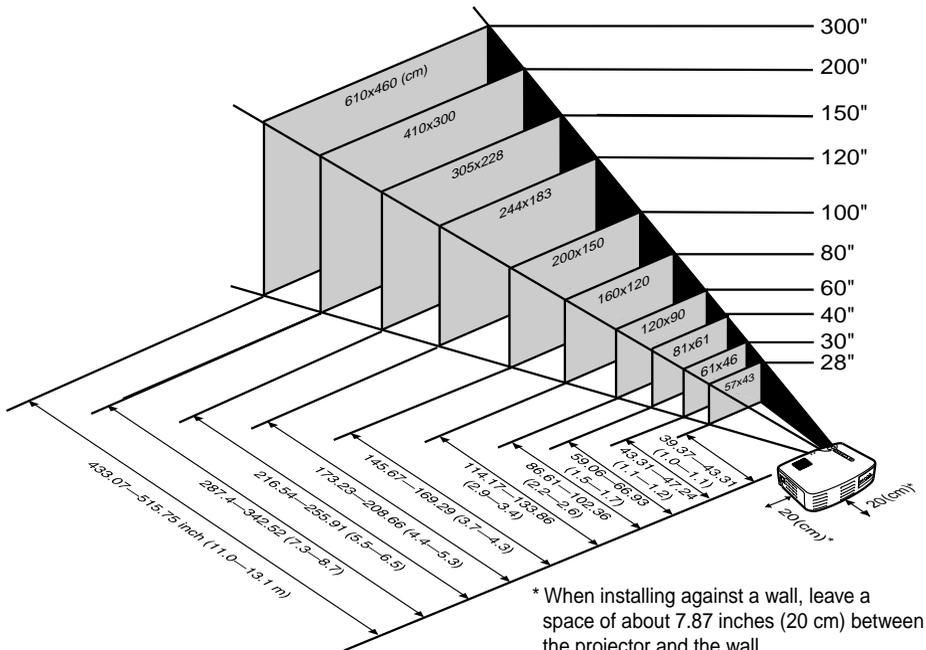
\* When installing against a wall, leave a space of about 7.87 inches (20 cm) between the projector and the wall.
