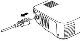
1. Switch off power to the projector and disconnect the power cord after cool-down\* ends.
