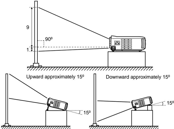
Keystone correction allows correction of trapezoidal distortion (See pages 29, 47).
