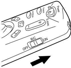
1. To use the remote control, turn the remote control R/C switch to "On".
