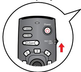
If using the remote control, set the R/C switch to the ON position and then press the
