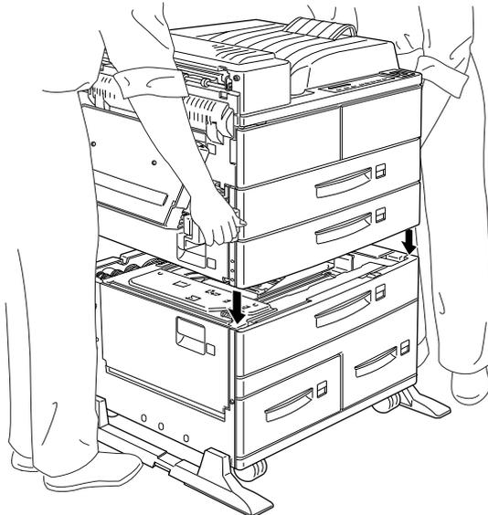
6. Make sure all corners of the printer fit firmly onto the unit.
