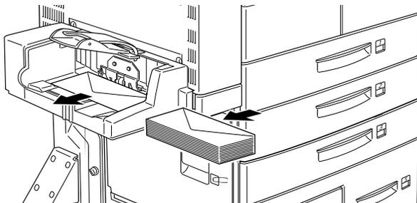
2. Tap the edges of the envelope stack on a flat surface. Then reload the envelopes in the envelope tray, making sure they are evenly aligned and rest below the maximum paper mark.
