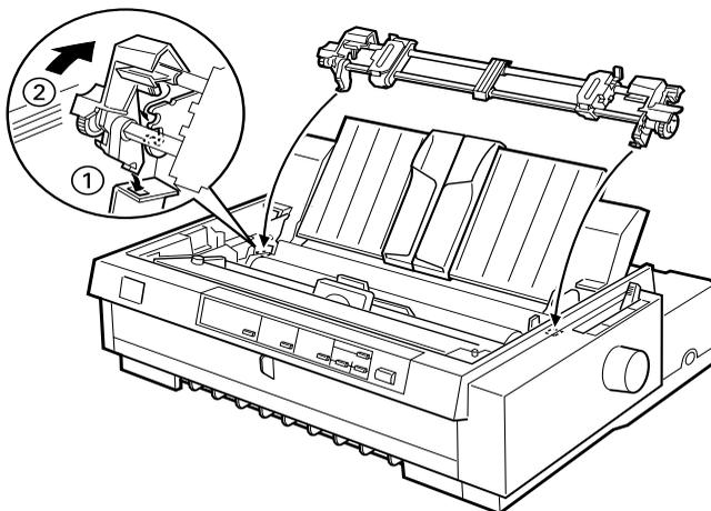
You are now ready to load continuous paper onto the pull tractor as described in the next section. To remove the pull tractor, see “Removing the pull tractor” on page 2-31.
