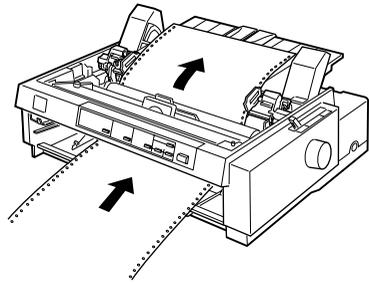
Load paper in the bottom slot printable side up (forward).
