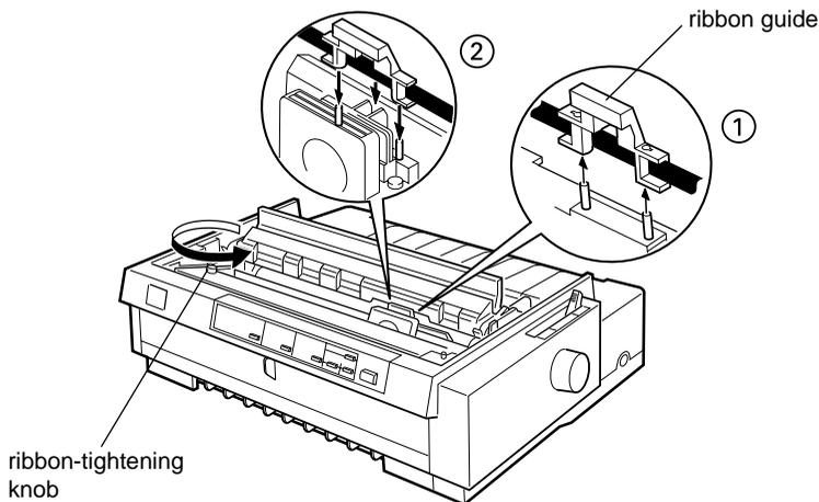
10. Turn the ribbon-tightening knob in the direction of the arrow to remove any slack in the ribbon as shown in step 9. Then slide the print head from side to side to make sure it moves smoothly.
