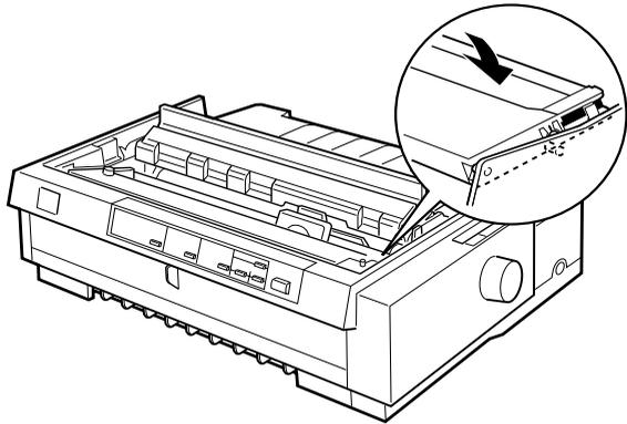
9. Lift the cartridge's ribbon guide (①) and insert it firmly over the metal pins behind the print head (②). Make sure the ribbon is not twisted or creased and that it is in place behind the print head. Then press down the guide until it clicks into place.
