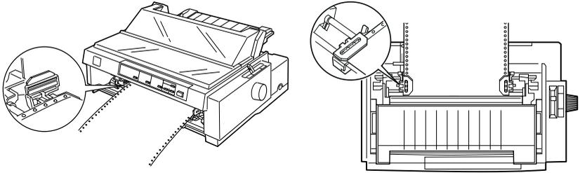
In the standby position, your paper is attached to the printer but is not inside the printer.
