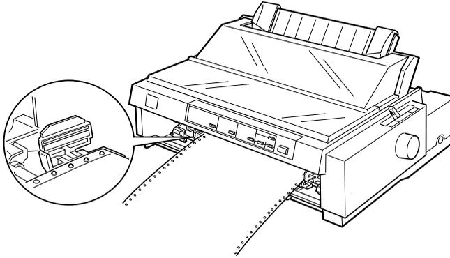
8. Slide the right sprocket to remove any slack in the paper; then lock it in place by pushing the sprocket lock down.
