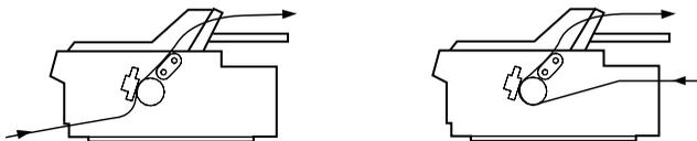
13. After you finish printing, open the paper guide cover; then tear off the printed document at the perforation nearest the paper exit slot.
