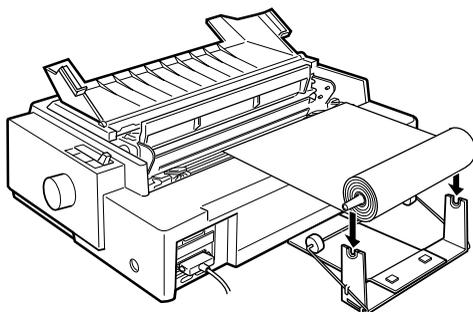
8. Turn on the printer. Bring the leading edge of the paper up over the rear push tractor and insert it until it meets resistance. The printer loads the roll paper automatically.
