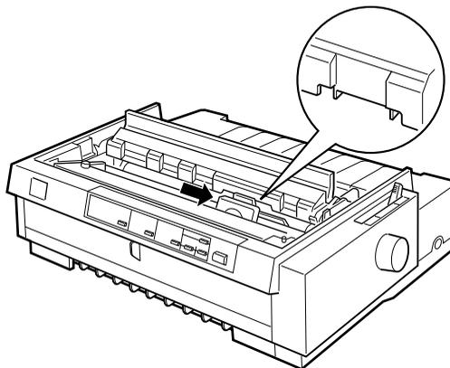
5. If a used ribbon cartridge is installed, grasp it the cartridge and pull it slightly forward and up; the ribbon guide snaps away from the metal pins behind the print head. Properly dispose of the used ribbon cartridge.
