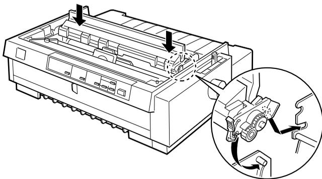
6. Replace the paper guide base and the printer cover. Then close the paper guide cover.
