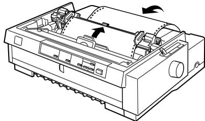
9. Fit three holes on each side of the paper over the tractor pins on both sprockets. Then close the sprocket covers.
