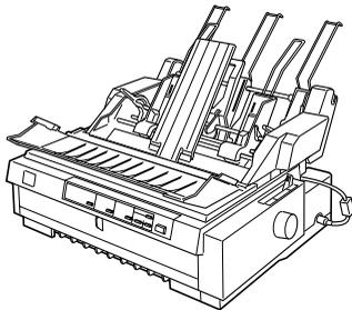
Connects to the high-capacity cut-sheet feeder to create a double-bin cut-sheet feeder. You can load up to 50 sheets of ordinary single-sheet paper in the second-bin cut-sheet feeder. See “Using the Optional Cut-Sheet Feeders” on page A-4 for instructions.
