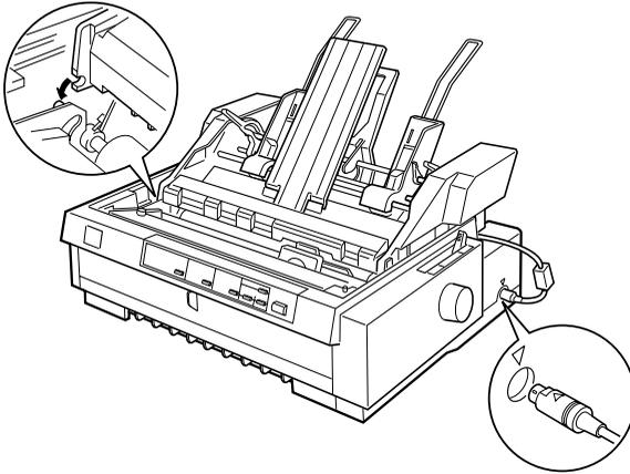
5. Insert the cable into the connector as shown above.
