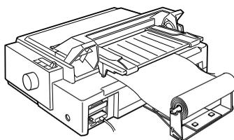
Allows you to use your printer with 8.5-inch roll paper like that used with telex machines. See “Using the Roll Paper Holder” on page A-13 for instructions.
