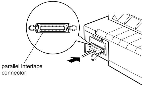
Squeeze the wire clips together until they lock in place on both sides of the connector.
