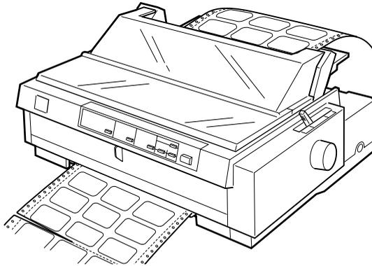
2. Hold down the LF/FF button to eject the remaining labels from the printer.
