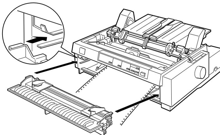
12. If you use the rear slot, replace the paper guide base and make sure the edge guides are together in the middle of the paper guide base and lift the center section of the paper guide base up and lay it flat.
