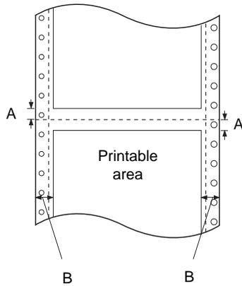
A The minimum top and bottom margins above and below the perforation are 4.2 mm each.
