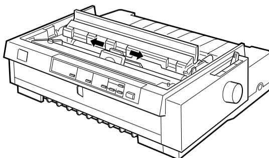
11. Replace the printer cover by first inserting the front tabs into the slots on the printer and then lowering the cover into place. Push it down until it clicks.
