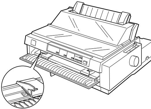
4. Set the paper release lever to the single-sheet position. Also set the paper thickness lever (located under the printer cover) to the proper position for your paper's thickness. (See the table on page 3-3.)
