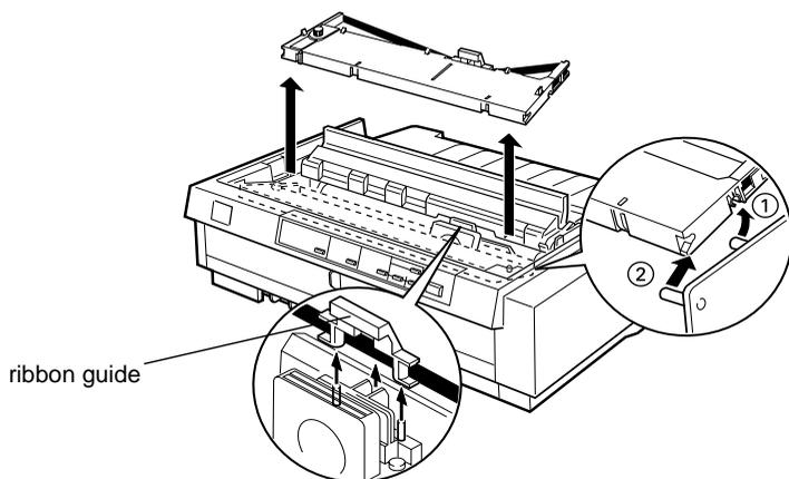
6. Remove the new ribbon cartridge from the package. Then remove the separator from the middle of the ribbon cartridge and discard the separator. Turn the ribbon-tightening knob in the direction of the arrow to remove any slack in the ribbon.
