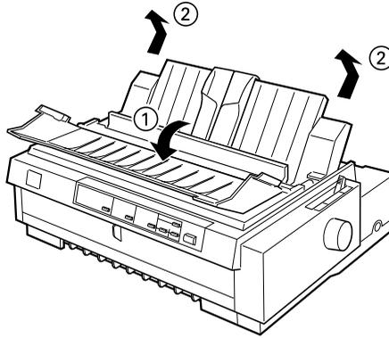
3. Set the paper release lever to the rear push tractor position. Set the paper thickness lever (located under the printer cover) to the proper position for your paper's thickness.
