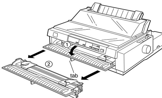
3. Insert the tractor into the printer's mounting slots and press down both ends of the tractor to make sure that it is firmly seated.
