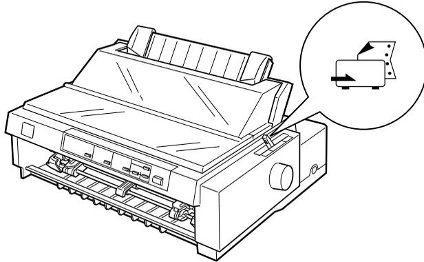
4. Release the left and right sprockets by pushing the sprocket lock levers backward.
