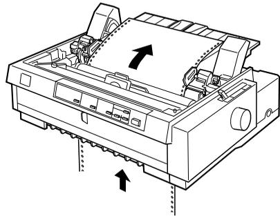
Before you load paper in the rear slot, remove the paper guide base. Then load paper in the rear slot, printable side down and attach the paper guide base.
