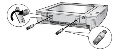
3. Place the two knobs included with the ADF beside the scanner.
