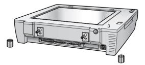
4. Slide the ADF onto the scanner, lining up the screws with the holes as shown.
