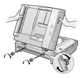
6. Attach the ADF's connector to the scanner's option interface. Then tighten the connector screws.
