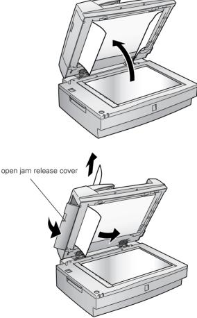
3. If paper jams in the paper eject position, open the cover on the right and slowly pull out the jammed paper as shown. (Be careful not to pull too hard or the paper may tear, making it more difficult to remove.)
