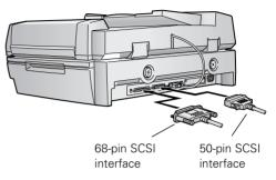
3. Connect the pin end of the SCSI cable to the SCSI port on your computer or another SCSI device in the chain and tighten the screws to secure the cable.
