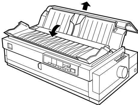
2. Set the paper release lever to the rear push tractor position. Also set the paper thickness lever (located under the printer cover) to the proper position for your paper's thickness.
