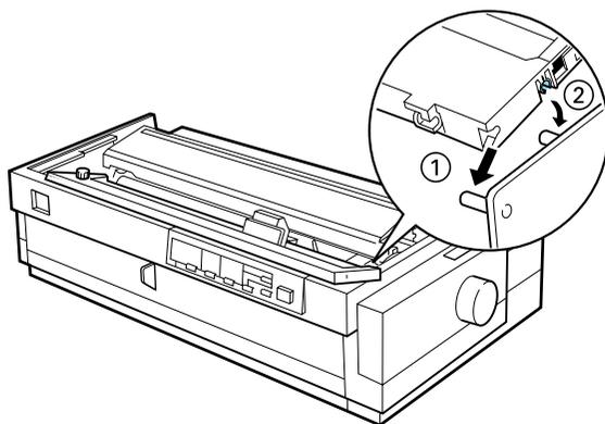
8. Make sure that the two rear notches of the cartridge fit over the small pegs on each side of the printer. Then gently press down the cartridge until both ends click into place.
