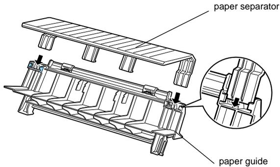
2. Make sure the paper guide cover is open as shown below. Attach the paper guide by sliding the slots on the bottom of the paper guide over the pegs behind the paper tension unit.
