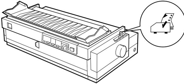
3. Release the left and right sprockets by pulling the sprocket lock levers forward.
