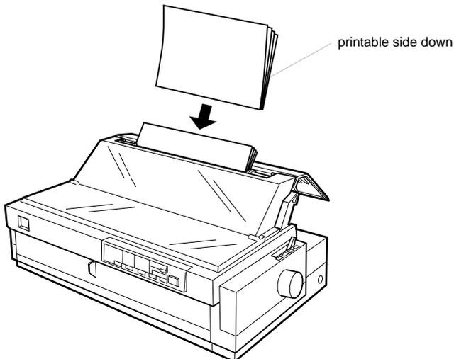
Insert this type of form in the front slot with the bound edge first and the printable side up, as shown below.
