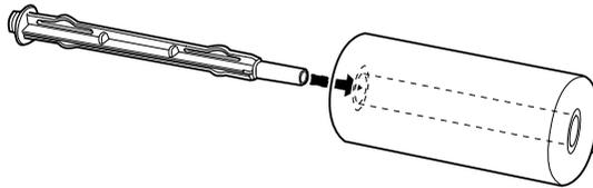
7. Place the shaft and paper roll on the roll paper holder so the paper feeds from the bottom of the roll.
