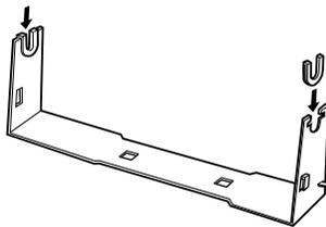
2. Make sure you orient the stand and base plate as shown below. Then place the base plate on the stand and fasten the two together with the plastic spacing clips.
