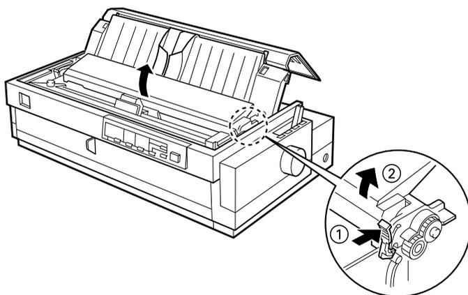
3. Lower the tractor into the printer's mounting slots and press down both ends of the tractor to make sure that it is firmly seated.
