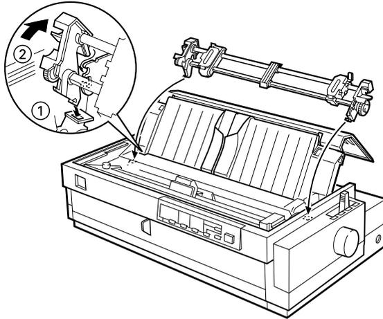
You are now ready to load continuous paper onto the pull tractor as described in the next section. To remove the pull tractor, see page 2-30.
