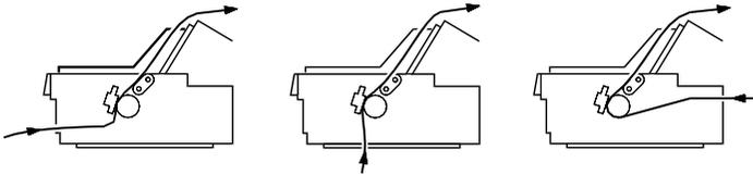
16. After you finish printing, open the paper guide cover; then tear off the printed document at the perforation nearest the paper exit slot.
