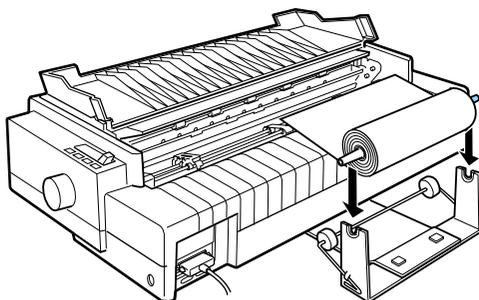
8. Turn on the printer. Then bring the leading edge of the paper up over the rear push tractor and insert it until it meets resistance. The printer loads the roll paper automatically.
