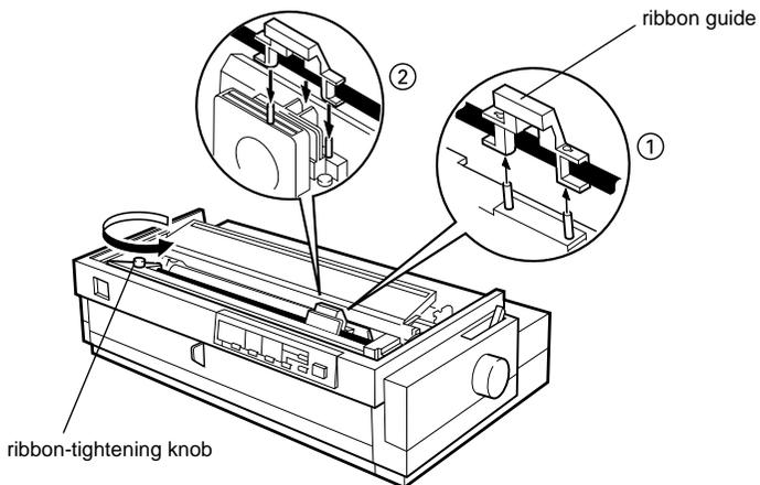
10. Turn the ribbon-tightening knob in the direction of the arrow to remove any slack in the ribbon, as shown above. Then slide the print head from side to side to make sure it moves smoothly.
