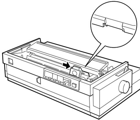
5. If a used cartridge is installed, grasp the cartridge and pull it slightly forward and up; the ribbon guide snaps away from the metal pins behind the print head. Properly dispose of the used ribbon cartridge.
