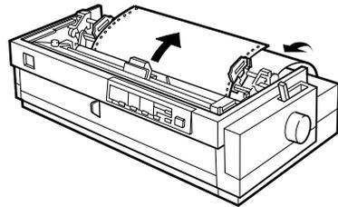
9. Fit four holes of the paper over the tractor pins on both sprockets. Then close the sprocket covers.
