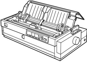
Improves continuous paper handling and reduces the chance of paper jams. You can also use this tractor as a front push tractor. Using a pull tractor in combination with a push tractor is especially useful for printing on continuous pre-printed forms, multipart forms, and labels, and for printing high-quality graphics. For instructions on using this option, see pages 2-10 and 2-27.
