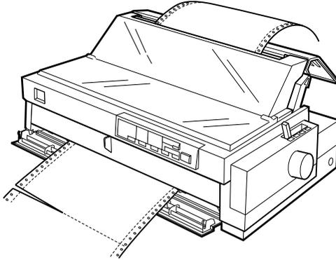
2. Hold down the LF/FF button to eject the paper from the printer.
