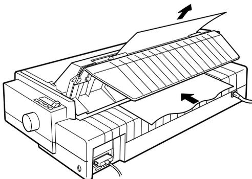
When you finish printing, open the paper guide cover and press the LF/FF button to advance the paper. Then tear off the paper using the tear-off edge of the printer (pull it towards you for a clean cut).
