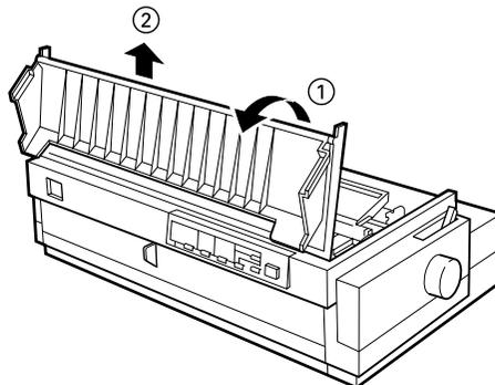
4. Make sure that the print head is not hot; if it is, let it cool for a few minutes before touching it. Then slide the print head to the ribbon installation position (the indented portion of the paper tension unit) by hand.
