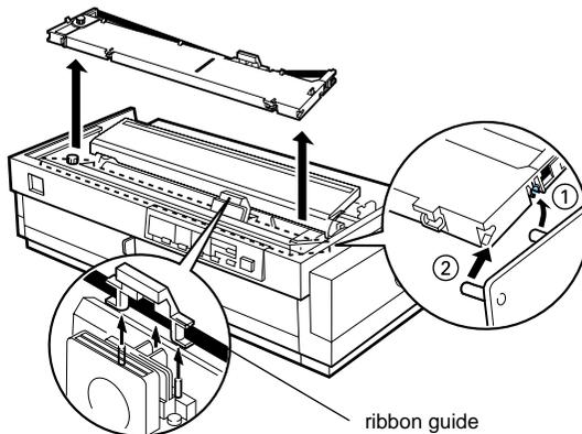
6. Remove the new ribbon cartridge from the package. Remove the separator from the middle of the ribbon cartridge and discard the separator. Then turn the ribbon-tightening knob in the direction of the arrow to remove any slack in the ribbon.
