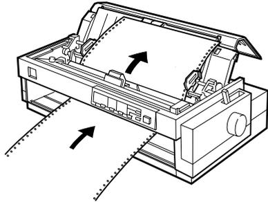
Load paper in the bottom slot printable side up (forward).
