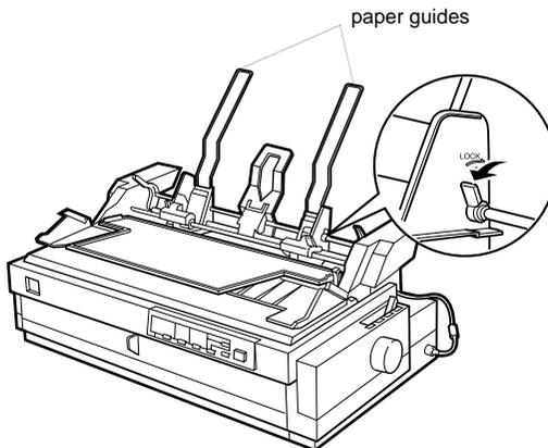
4. Holding the lower portion of the left paper guide, slide it until it is aligned with the arrow mark on the back of the center support. Then push the left lock lever backward to lock it in place. Holding the lower portion of the right paper guide, slide it to match the width of your paper, but do not lock it.
