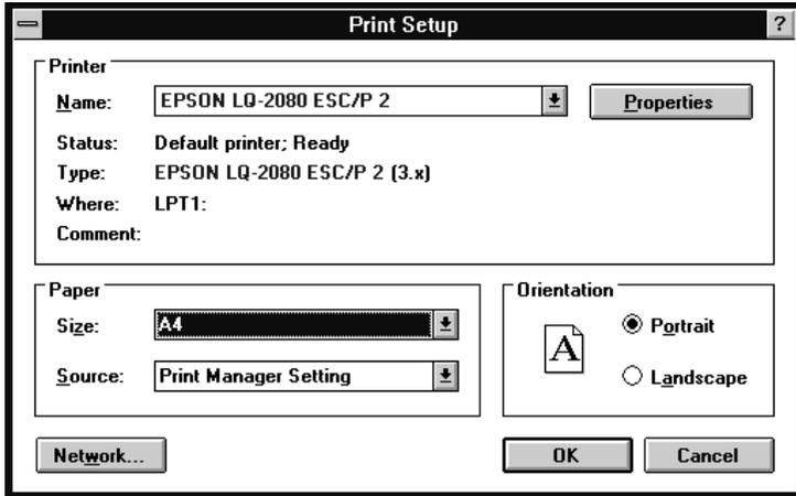
2. Make sure that your printer is selected and then click Printer, Setup, Properties, or Options. (You may need to click a combination of these buttons.) The screen displays the Document Properties dialog box, which contains the Form and Orientation printer driver settings. See "Printer driver settings overview" on page 4-20 for detailed information about these settings.
