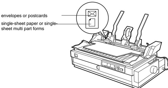
7. Pull both paper set levers forward until the paper guides retract and lock open to allow paper loading.
