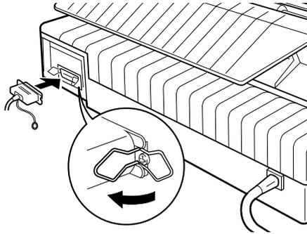
3. If your cable has a ground wire, connect it to the printer's ground connector as shown below.
