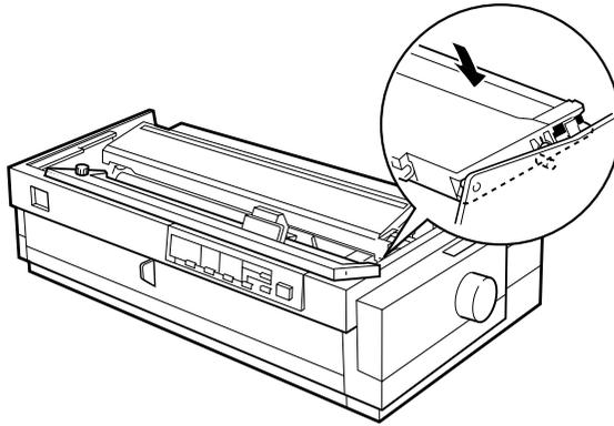
9. Lift the cartridge's ribbon guide (①) and insert it firmly over the metal pins behind the print head (②). Make sure the ribbon is not twisted or creased and that it is in place behind the print head. Then press down the guide until it clicks into place.
