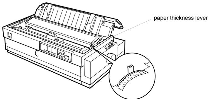
Use the following table to set the paper thickness lever to match the thickness of your paper.
