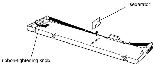
7. Hold the cartridge with the ribbon-tightening knob up. Fit the two front notches of the ribbon cartridge over the small pegs on each side of the printer as shown below. Then lay the cartridge flat.
