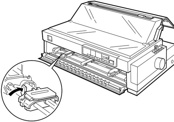
4. Slide the left sprocket to the left margin of your paper using the arrow mark inside the printer. (Printing starts at the arrow mark.) Then pull the lever forward to lock it in place.
