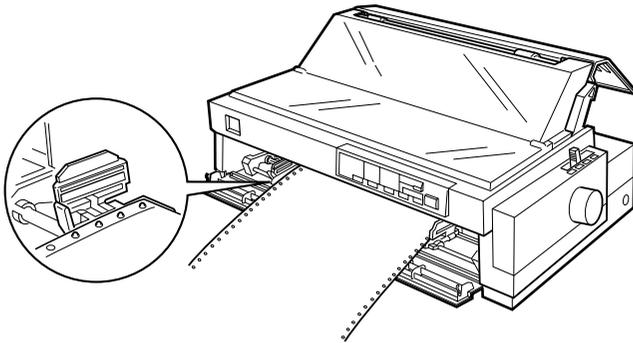
7. Slide the right sprocket to remove any slack in the paper; then lock it in place by pushing the sprocket lock down.
