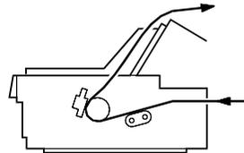
12. After you finish printing, open the paper guide cover; then tear off the printed document at the perforation nearest the paper exit slot.
