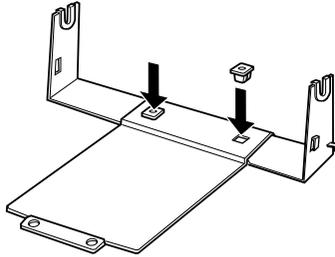
3. Hook the tension lever onto both ends of the stand as shown below. While pulling up the tension lever, fit the wire ends of the tension lever into the holes in the stand. The roll paper holder is assembled.
