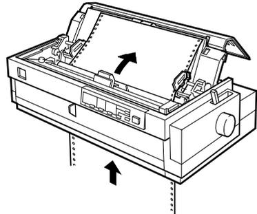
Before you load paper in the rear slot, remove the paper guide. Then load paper in the rear slot printable side down.
