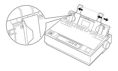
4. Slide a sheet of paper down firmly between the edge guides until it meets resistance. The printer loads the sheet automatically. Press the PAUSE button, then the printer begins to print.
