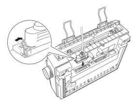
2. Guide the interface cable through the slot on the side of the printer so that it does not block the paper supply as shown in the illustration on page 1-16.
