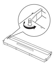
4. Insert the ribbon cartridge into the printer as shown; then press both sides of the cartridge firmly to fit the plastic hooks into the printer slots.
