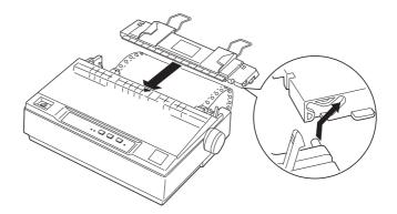
6. Slide the left edge guide to the center until it stops at the guide mark. Then slide the right edge guide to the opposite guide mark.
