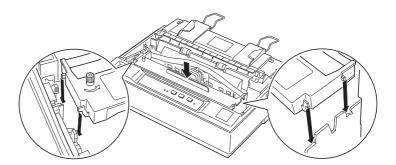
5. Use a pointed object, such as a ball point pen, to guide the ribbon between the print head and ribbon guide. Turn the ribbon tightening knob to help feed the ribbon into place; it should not be twisted or creased.
