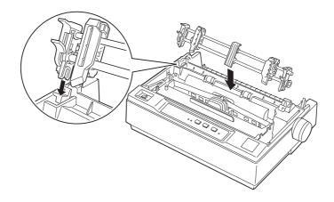
4. Release the sprocket units by pulling the sprocket locks forward.
