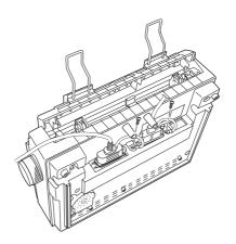
2. Guide the interface cable through the slot on the side of the printer so that it does not block the paper supply.
