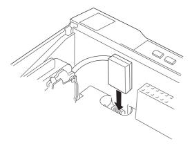
4. Slide the print head to the middle of the printer; then slide the plastic part on the color ribbon to the center of the cartridge.
