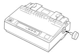
2. Push firmly on the paper-feed knob until it fits against the printer case.
