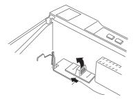
2. Install the motor unit in the right hand corner of the printer, with the gear facing the center of the printer. Push it down firmly to fit the metal pins into the slots.
