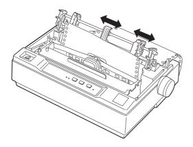
7. Make sure your paper has a clean, straight leading edge. Open the sprocket covers. Fit the first holes of the paper over the sprocket pins and then close the sprocket covers. Slide the right sprocket unit to remove any slack in the paper and lock it in place.
