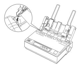
5. Slide the left paper guide so it is aligned with the triangle mark. Next, slide the right paper guide to roughly match the width of your paper. Slide the paper support midway between the paper guides.
