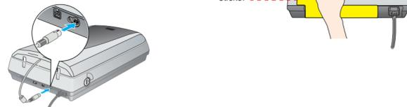
4 Connect either the USB cable that came with the scanner or an optional IEEE 1394 (FireWire) cable. **Do not connect both cables.**
