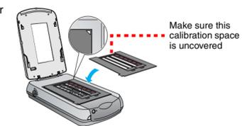
If you are scanning slides, place the holder on the scanner. Then place the slides in the holder.
