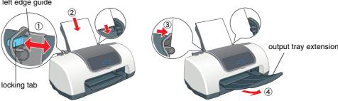
To adjust the left edge guide, hold down the locking tab and slide the guide against the paper stack
