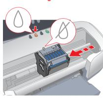
3. Then, press the  $\Diamond$  ink button again. The print head moves to the ink cartridge replacement position.
