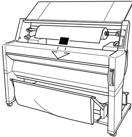
6. Pull the paper down through the paper insertion slot a small way.
