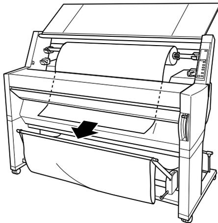
7. Roll back the roll paper to remove the slack. Make sure that the bottom edge of the paper is positioned straightly and in line with the rows of punch holes.
