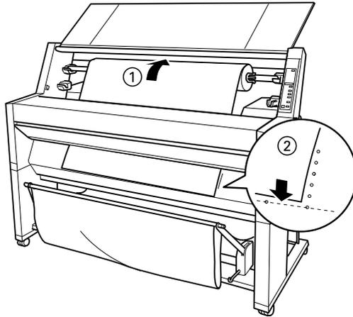
8. Push the paper set lever all the way down, then close the roll paper cover. `PRESS PAUSE BUTTON` appears.
