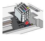
Install all ink cartridges. This product does not work unless all cartridges are installed properly
