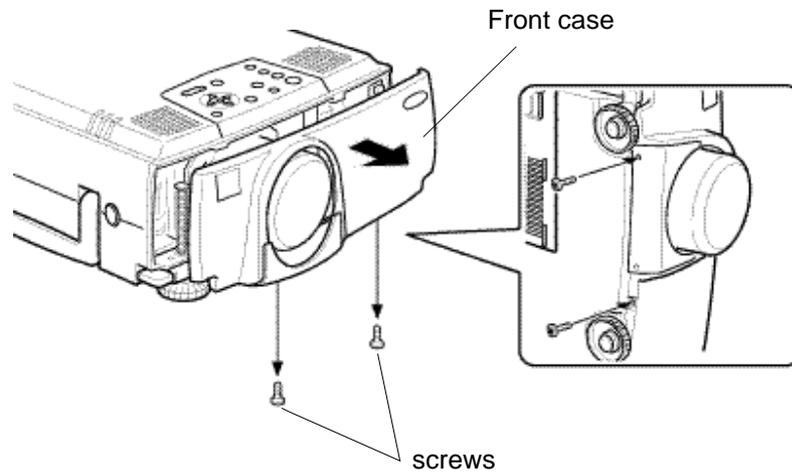
(2) Unscrew the four screws to remove the existing lens using a hexagon head screwdriver supplied with the long zoom lens.
