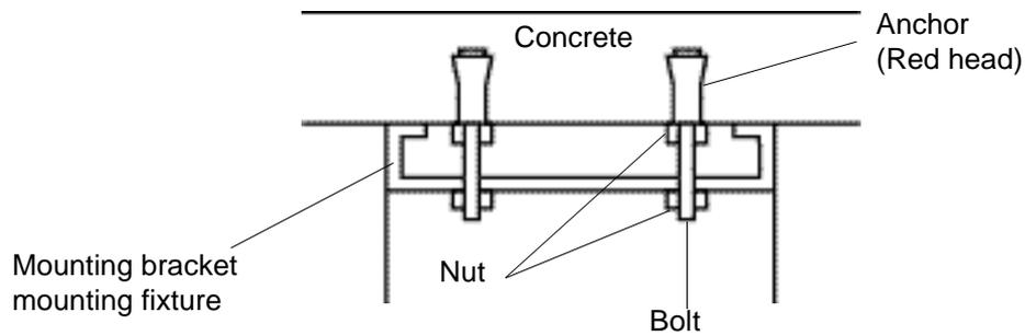
(2) Mount the ceiling mounting bracket using common nuts (available in stores).
