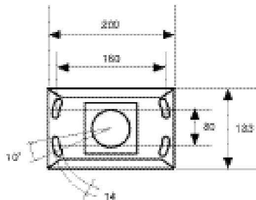
First, mount only the ceiling mounting bracket. Then the assembled adjustment bracket and projector may be installed.
