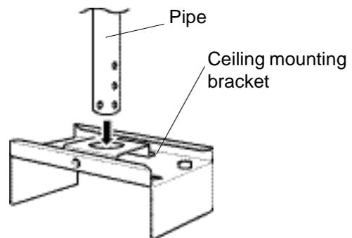
(2) Mount the ceiling mounting bracket catch as shown below and secure with the catch set-bolt and nut.
