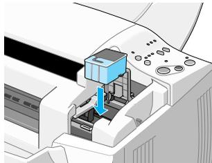
6. Press the ink cartridge clamp down until it locks into place. The
