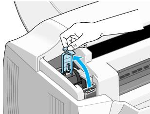
9. When installation is complete, press the
