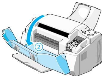
2. Turn on the Stylus Scan by pressing its
