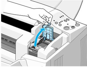
4. Open the color ink cartridge package that came with your Stylus Scan. Remove only the yellow tape seal from the ink cartridge.
