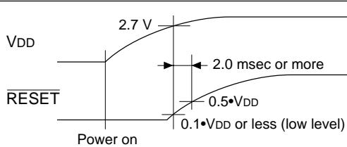
E0C63P366 uses the initial reset signal as a trigger for setting either the normal operation mode or the programming mode. Therefore, design the reset input circuit so that the IC will be reset for sure. Initial resetting during operation is the same as the E0C63158.
