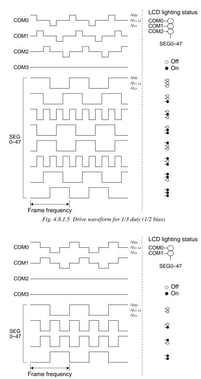
Fig. 4.8.1.6 Drive waveform for 1/2 duty (1/2 bias)
