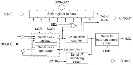
Fig. 4.7.1.1 Configuration of serial interface
