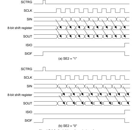
Fig. 4.7.3.2 Serial interface timing chart
