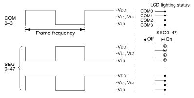
Fig. 4.8.2.2 Drive waveform for 1/1 duty (1/2 bias)
