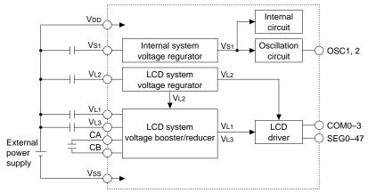
Fig. 2.1.1 Power supply configuration of E0C6008
