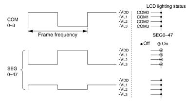
Fig. 4.8.2.1 Drive waveform for 1/1 duty (1/3 bias)
