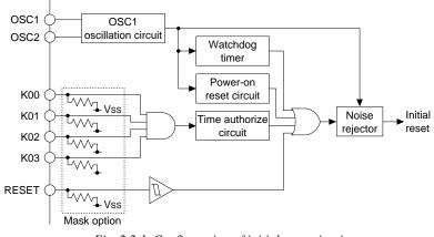
Fig. 2.2.1 Configuration of initial reset circuit
