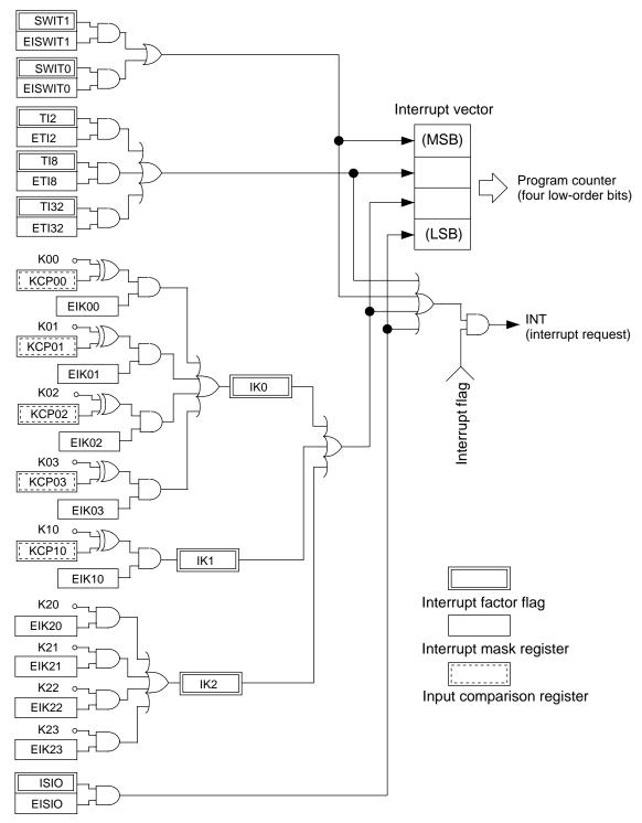
Fig. 4.16.1 Configuration of interrupt circuit
