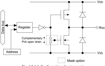
Fig. 4.5.1.1 Configuration of output ports
