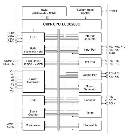
Fig. 1.3.1 Block diagram
