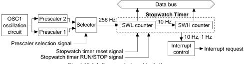
Fig. 4.10.1.1 Stopwatch timer block diagram
