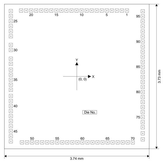
Chip thickness: 400µm Pad opening: 95µm
