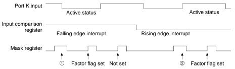
When the content of the mask register is rewritten while the port K input is in the active status, the input interrupt factor flags are set at ① and @, ① being the interrupt due to the falling edge and @ the interrupt due to the rising edge.
