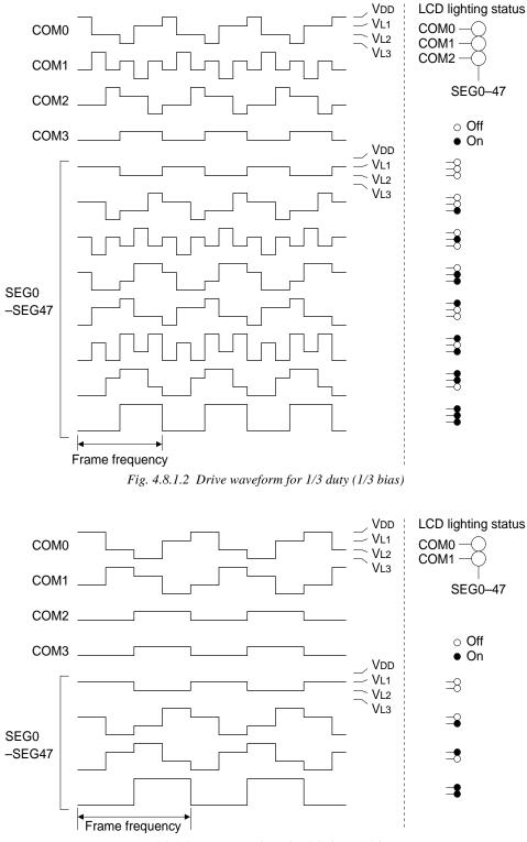
Fig. 4.8.1.3 Drive waveform for 1/2 duty (1/3 bias)
