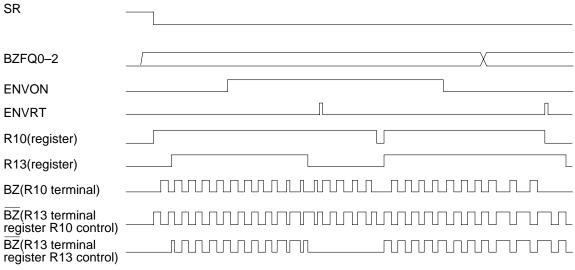
Fig. 4.11.1.2 Timing chart of sound generator
