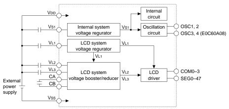
Fig. 2.1.2 Power supply configuration of E0C60A08 and E0C60L08
