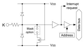
Fig. 4.4.1.1 Configuration of input port
