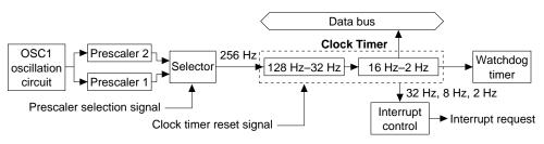
Fig. 4.9.1.1 Clock timer block diagram
