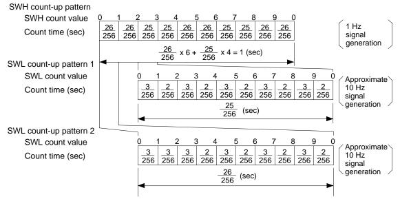
Fig. 4.10.2.1 Count-up pattern of stopwatch timer
