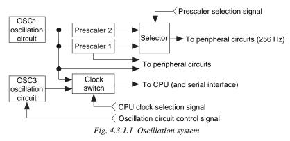
As Figure 4.3.1.1 indicates, two prescalers (demultiplier stage) are connected to the oscillation circuit. Prescaler 1 is for 32.768 kHz and prescaler 2 is for 38.4 kHz. These can be selected through the software to suit the crystal oscillator. This selection invokes the basic signal (256 Hz) for running the clock timer, stopwatch timer, and so forth.
