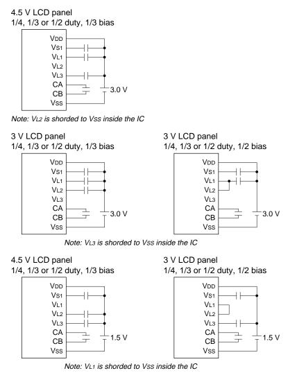
Fig. 2.1.3 External elements when LCD system voltage regulator is not used
