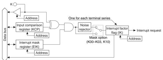
Fig. 4.4.2.1 Input interrupt circuit configuration (K00–K03, K10)
