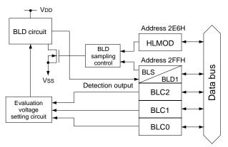
Fig. 4.14.1.1 Configuration of BLD circuit
