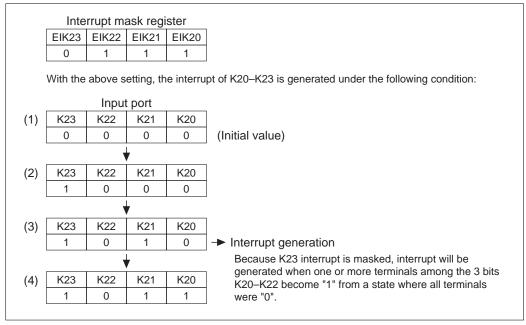
Fig. 4.4.2.4 Example of interrupt of K20–K23
