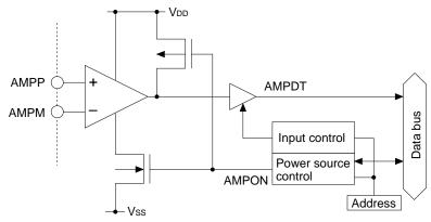
Fig. 4.13.1.1 Configuration of analog comparator
