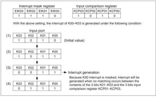
Fig. 4.4.2.2 Example of interrupt of K00–K03
