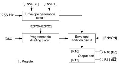
Fig. 4.11.1.1 Configuration of sound generator
