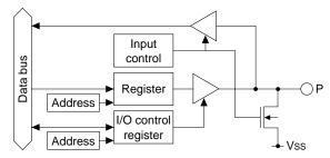
Fig. 4.6.1.1 Configuration of I/O port
