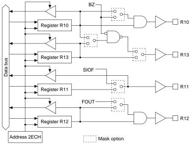
Fig. 4.5.2.1 Structure of output port R10-R13
