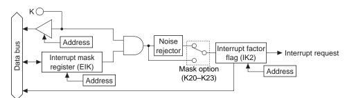
Fig. 4.4.2.3 Input interrupt circuit configuration (K20–K23)
