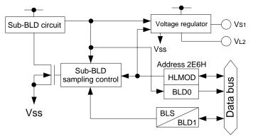
Fig. 4.15.1.1 Configuration of sub-BLD circuit
