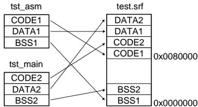
Fig. 3.4.1 Section allocation after linkage
