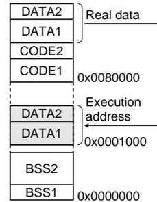
Fig. 12.7.1 Example of how data is located in a virtual section
