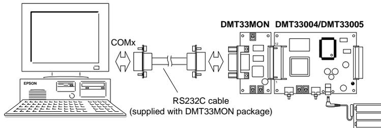
Fig. 16.8.1.4 Debugging system using DMT33004/DMT33005 board
