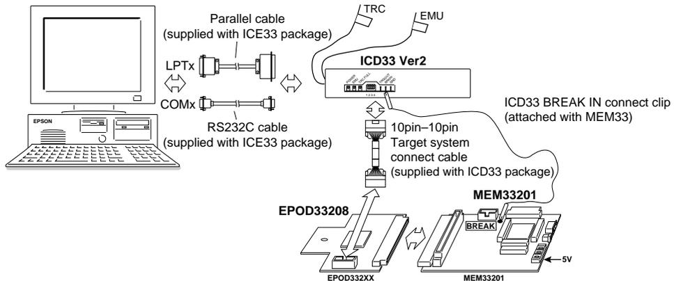
Fig.3.3.4.1 Debugging system using ICD33, EPOD33208, MEM33201
