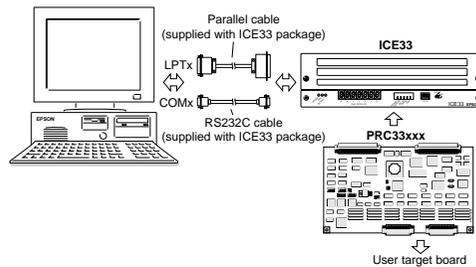
Fig. 3.3.1.1 Debugging system configuration using ICE33
