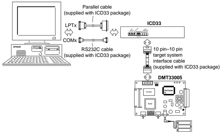
Fig. 16.8.1.2 Debugging system using ICD33 and DMT33005
