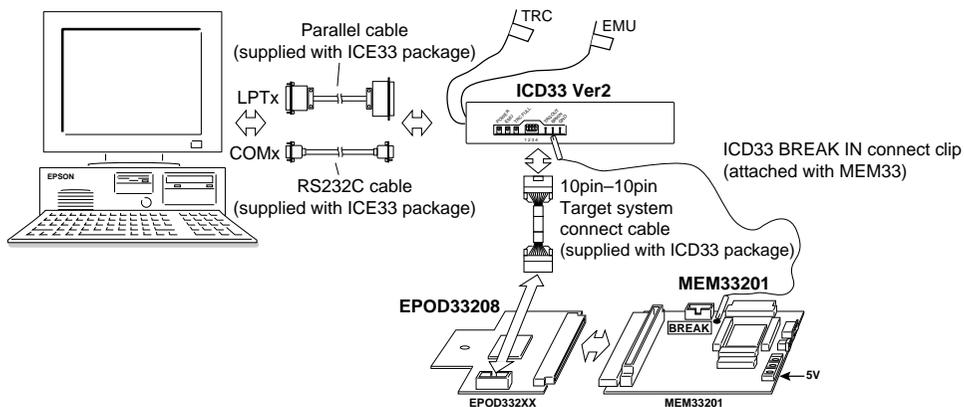
Fig. 16.8.1.3 Debugging system using ICD33, EPOD33208, MEM33201
