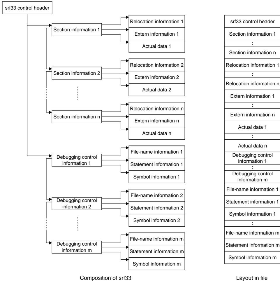
Fig. A.1 Structure of srf33 object file
