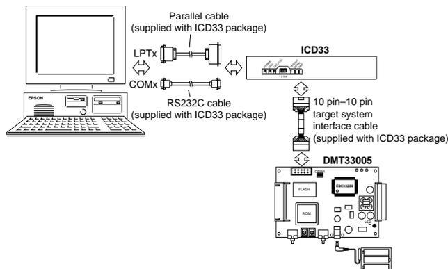
Fig. 3.3.3.1 Debugging system using ICD33 and DMT33005
