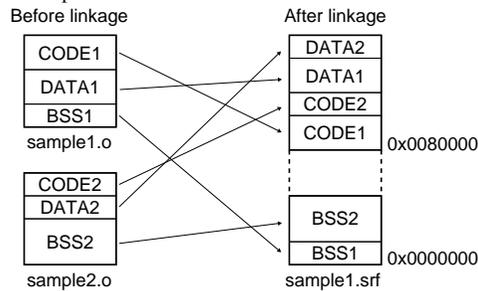
Fig. 12.6.1 Example of standard linkage
