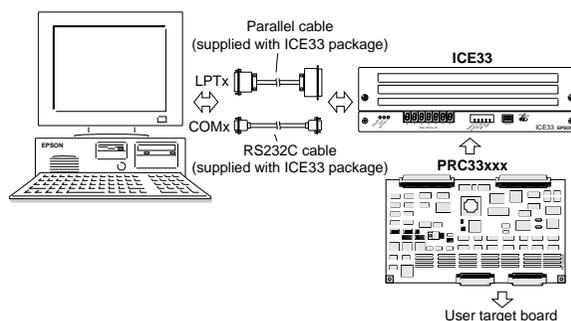
Fig. 16.8.1.1 Debugging system using ICE33
