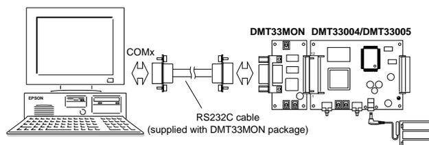
Fig. 3.3.2.1 Debugging system using DMT33004/DMT33005 board
