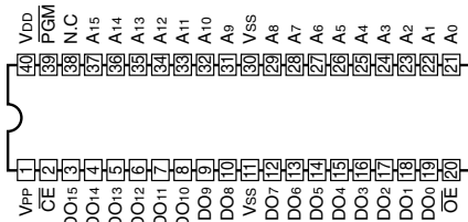
40-Pin DIP 1 Mbit Pin Arrangement
