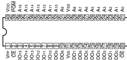
40-Pin DIP 2 Mbit Pin Arrangement
