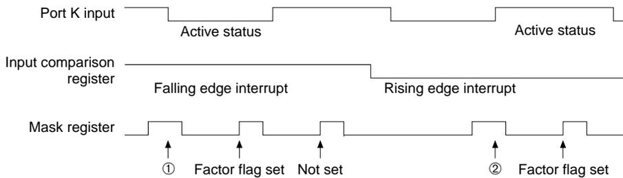
When the content of the mask register is rewritten while the port K input is in the active status, the input interrupt factor flags are set at ① and ②, ① being the interrupt due to the falling edge and ② the interrupt due to the rising edge.
