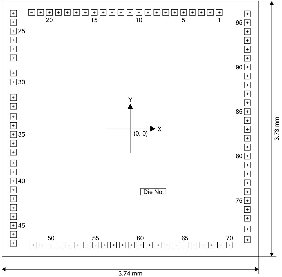
Chip thickness: 400 $\mu$ m
