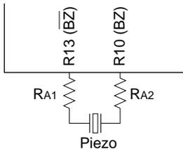
When the piezoelectric buzzer is driven directly
