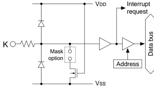
Fig. 4.4.1.1 Configuration of input port
