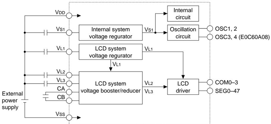
Fig. 2.1.2 Power supply configuration of E0C60A08 and E0C60L08
