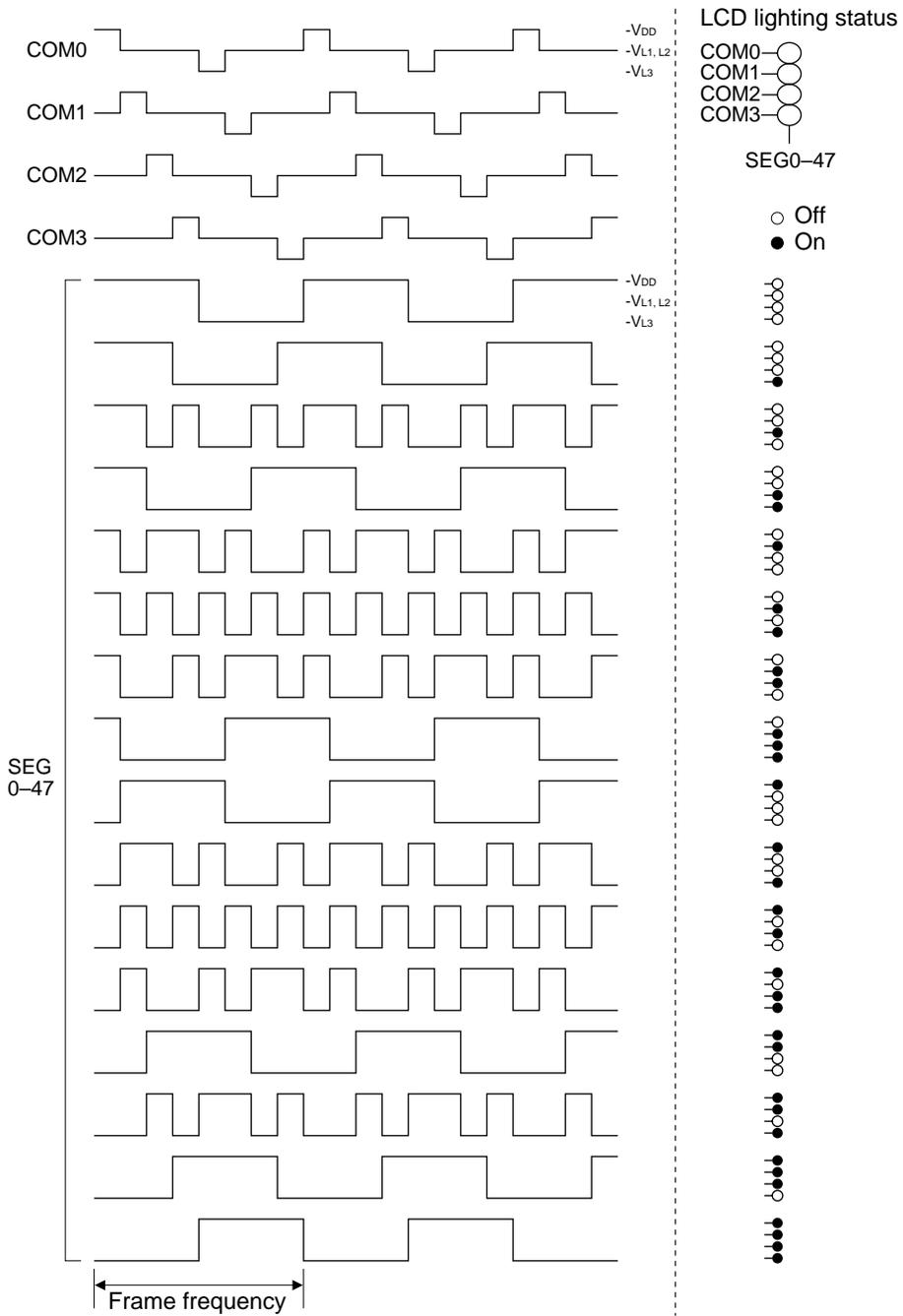
Fig. 4.8.1.4 Drive waveform for 1/4 duty (1/2 bias)
