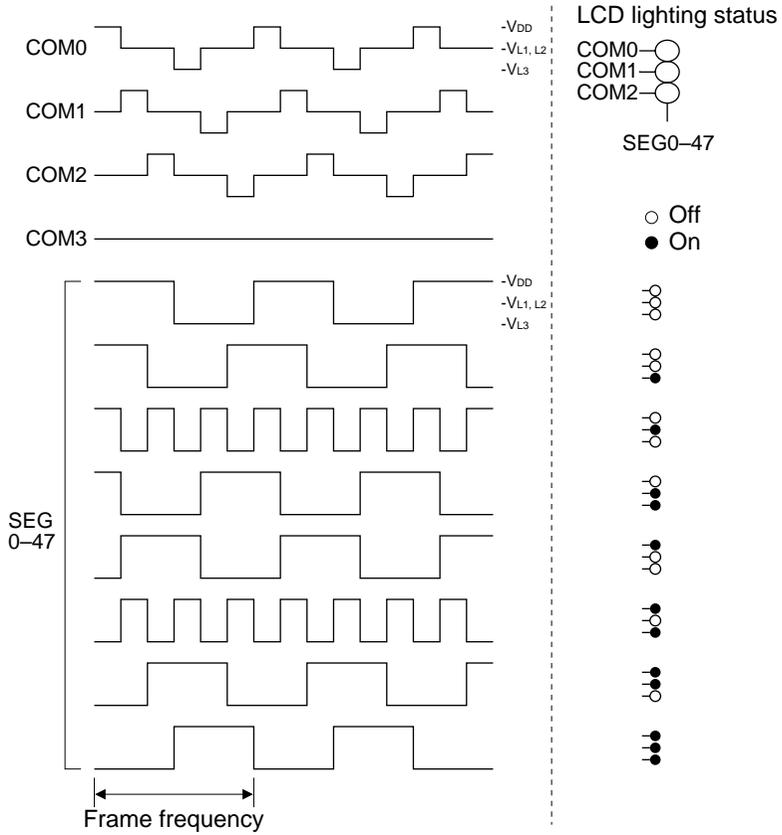
Fig. 4.8.1.5 Drive waveform for 1/3 duty (1/2 bias)
