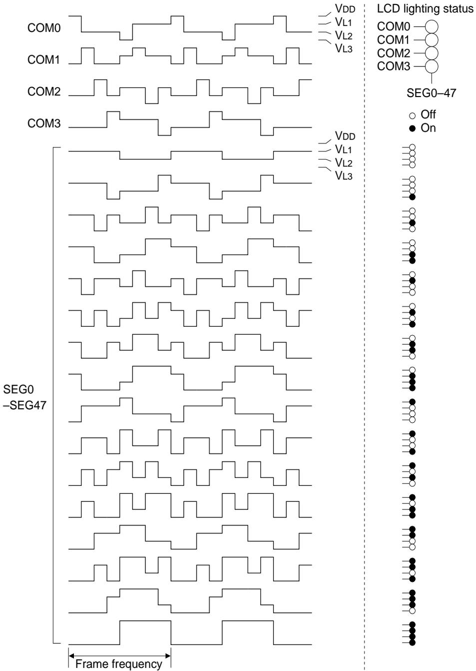
Fig. 4.8.1.1 Drive waveform for 1/4 duty (1/3 bias)
