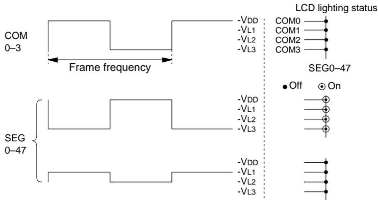
Fig. 4.8.2.1 Drive waveform for 1/1 duty (1/3 bias)
