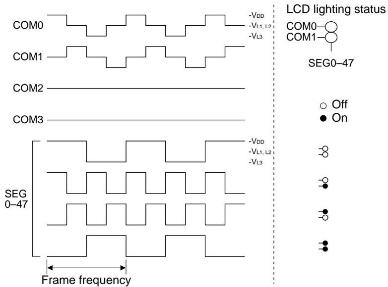
Fig. 4.8.1.6 Drive waveform for 1/2 duty (1/2 bias)
