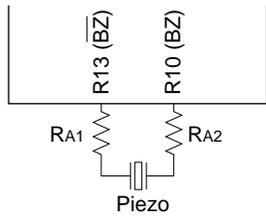
When the piezoelectric buzzer is driven directly
