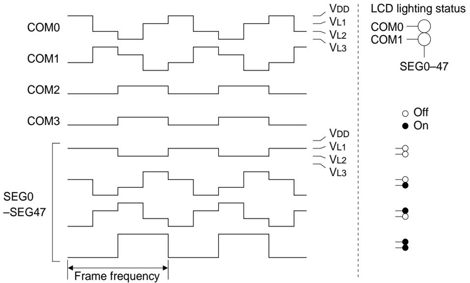
Fig. 4.8.1.3 Drive waveform for 1/2 duty (1/3 bias)
