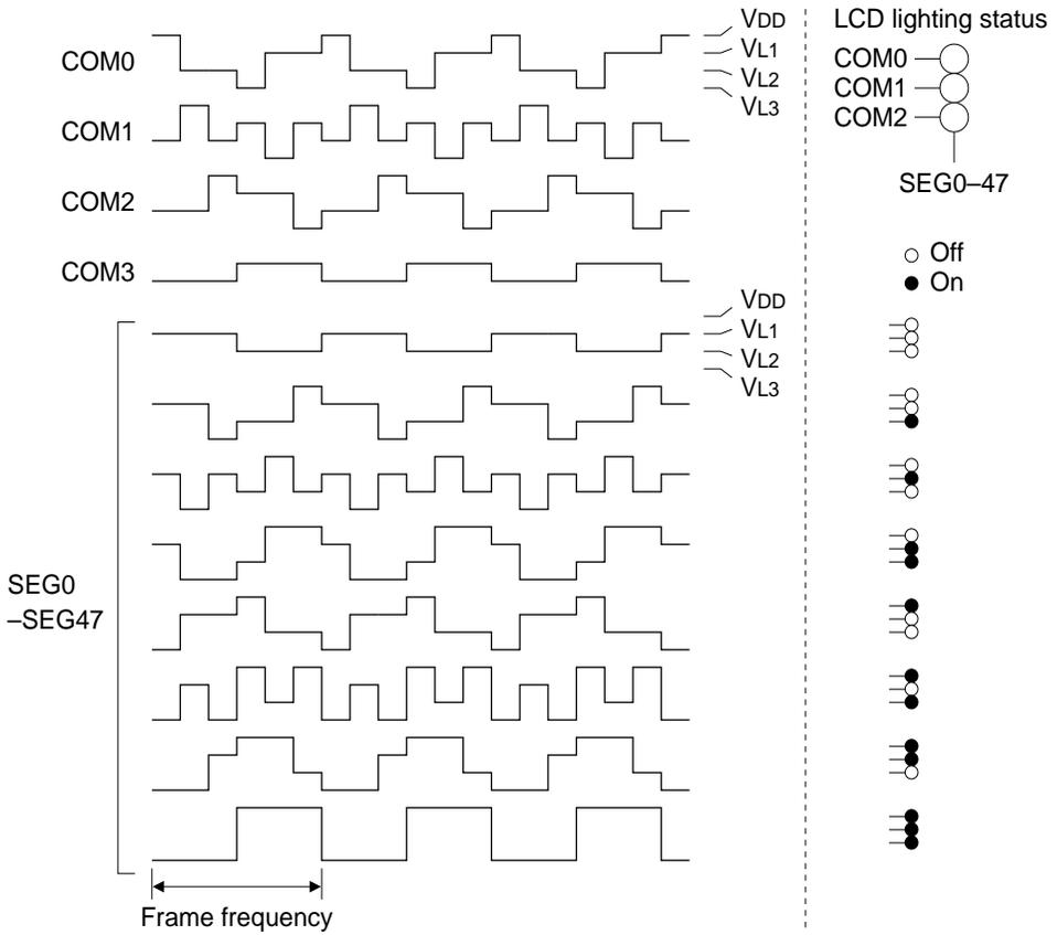
Fig. 4.8.1.2 Drive waveform for 1/3 duty (1/3 bias)
