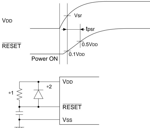
\*1 When the built-in pull up resistor is not used.
