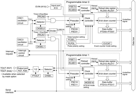
Fig. 5.10.1.1 Configuration of programmable timer
