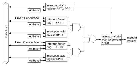
Fig. 5.10.7.1 Configuration of programmable timer interrupt circuit
