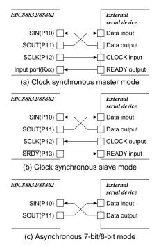
Fig. 5.7.3.1 Connection examples of serial interface I/O terminals
