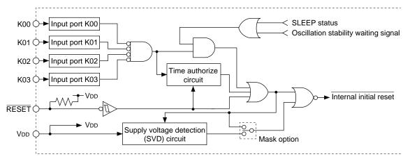
Fig. 4.1.1 Configuration of initial reset circuit
