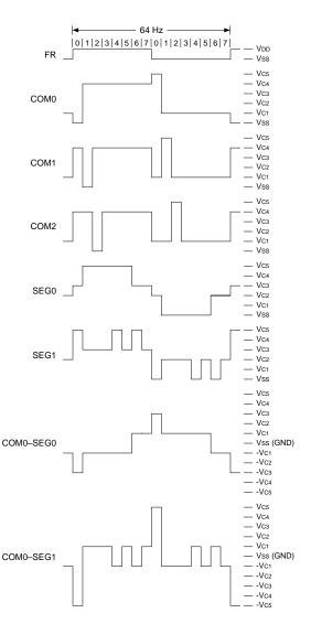
Fig. 5.11.4.3 Drive waveform for 1/8 duty
