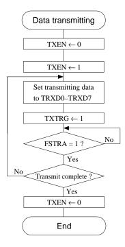
Fig. 5.7.7.2 Transmit procedure in asynchronous mode
