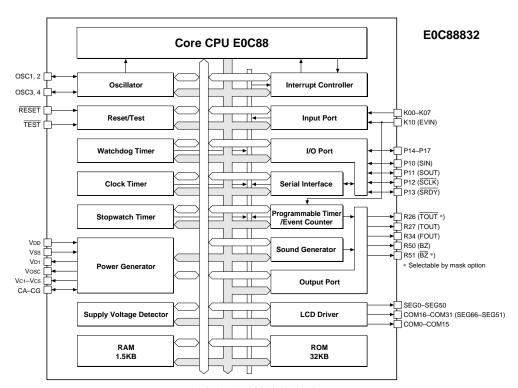
Fig. 1.3.1 E0C88832 block diagram
