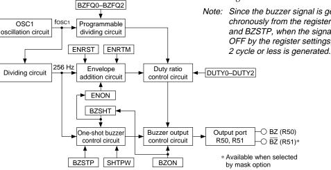
Fig. 5.12.1.1 Configuration of sound generator
