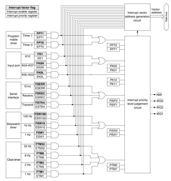
Fig. 5.14.1 Configuration of interrupt circuit
