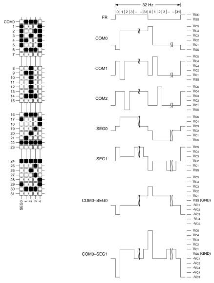
Fig. 5.11.4.1 Drive waveform for 1/32 duty
