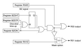
Fig. 5.5.5.5 Configuration of R50 and R51
