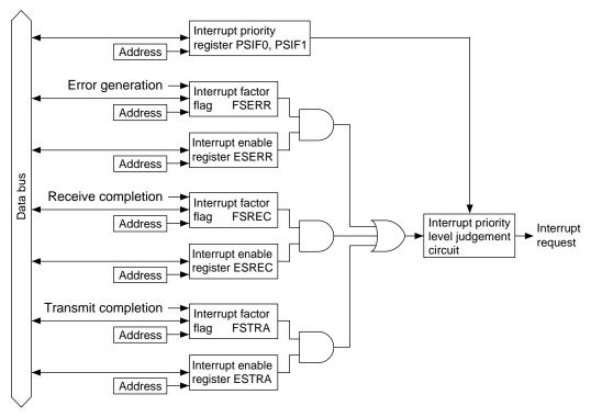
Fig. 5.7.8.1 Configuration of serial interface interrupt circuit
