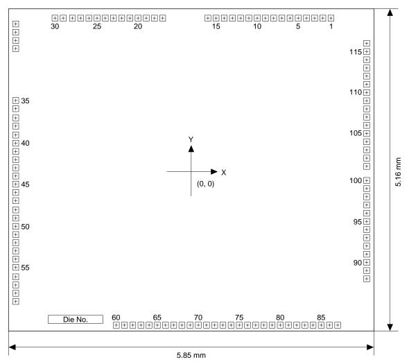
Chip thickness: 0.4 mm Pad opening: 100 μm
