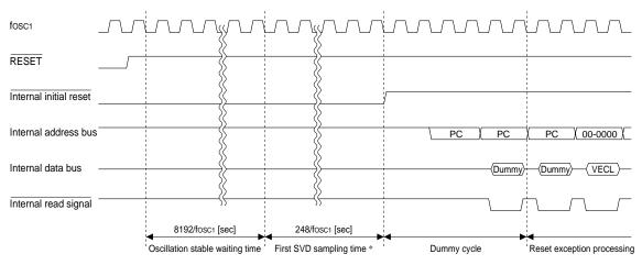
\* When the initial reset by the SVD circuit with the mask option has been used, this cycle is inserted as the waiting time.
