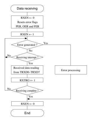
Fig. 5.7.7.3 Receiving procedure in asynchronous mode
