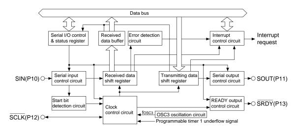
Fig. 5.7.1.1 Configuration of serial interface
