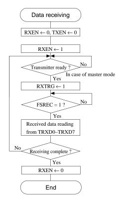
Fig. 5.7.6.3 Receiving procedure in clock synchronous mode
