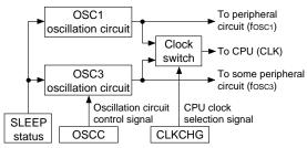
Fig. 5.3.1.1 Configuration of oscillation circuits
