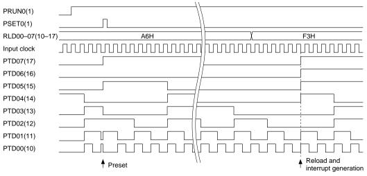
Fig. 5.10.2.1 Basic operation timing of the counter
