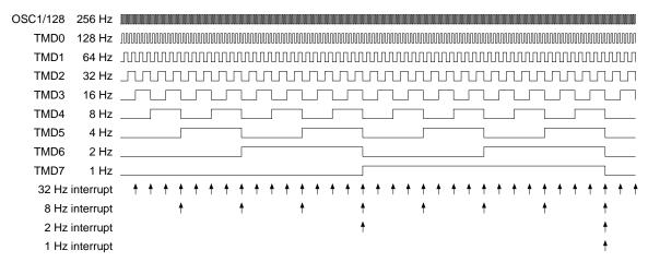
Fig. 5.8.2.2 Timing chart of clock timer
