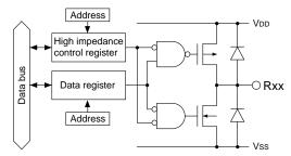
Fig. 5.5.1.1 Structure of output ports
