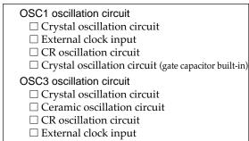
In terms of the oscillation circuit types for OSC1, either crystal oscillation, CR oscillation, crystal oscillation (gate capacitor built-in) or external clock input can be selected with the mask option. In terms of oscillation circuit types for OSC3, either crystal oscillation, ceramic oscillation, CR oscillation or external clock input can be selected with the mask option, in the same way as OSC1.
