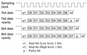
Fig. 5.7.7.1 Transfer data configuration for asynchronous system
