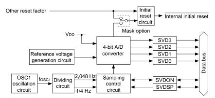
Fig. 5.13.1.1 Configuration of SVD circuit
