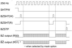
Fig. 5.12.5.1 Timing chart of one-shot output
