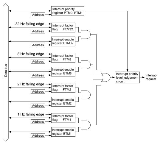
Fig. 5.8.2.1 Configuration of clock timer interrupt circuit
