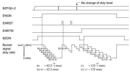
Fig. 5.12.4.1 Timing chart of digital envelope
