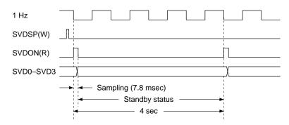
Fig. 5.13.2.2 Timing chart of 1/4 Hz auto-sampling
