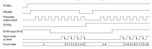
Fig. 5.10.6.1 Timing chart for pulse width measurement timer mode
