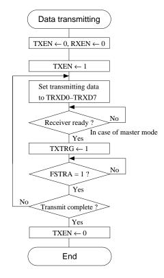
Fig. 5.7.6.2 Transmit procedure in clock synchronous mode
