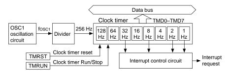
Fig. 5.8.1.1 Configuration of clock timer
