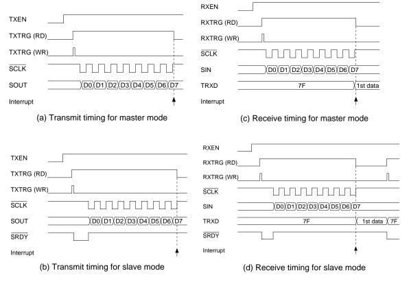
Fig. 5.7.6.4 Timing chart (clock synchronous system transmission)
