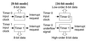
Fig. 5.10.2.3 8/16-bit mode setting and counter configuration
