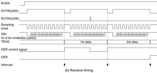
Fig. 5.7.7.4 Timing chart (asynchronous transfer)
