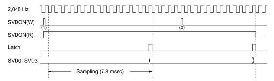
Fig. 5.13.2.1 Timing chart of continuous sampling
