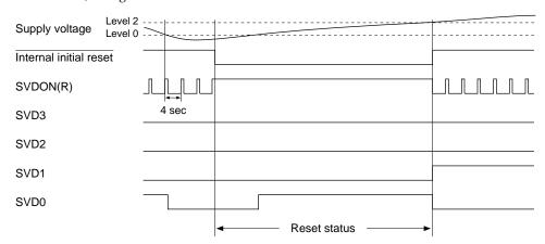
Fig. 5.13.2.3 Timing chart of the initial reset signal generation
