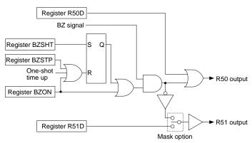
Fig. 5.12.2.1 Configuration of R50 and R51
