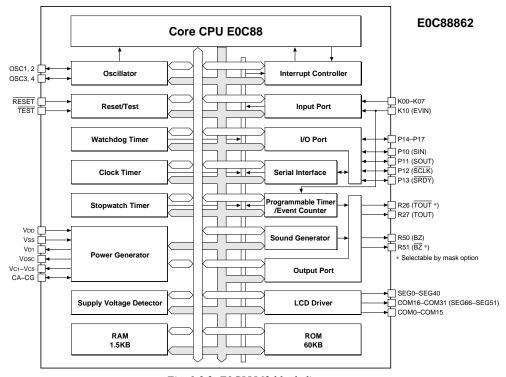
Fig. 1.3.2 E0C88862 block diagram
