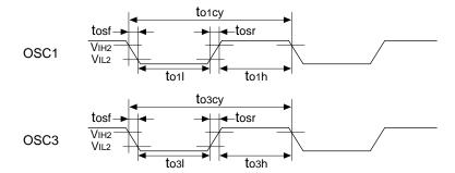
• SCLK, EVIN input clock (Normal operating mode) Condition: VDD = 2.4 to 5.5 V, Vss = 0 V, Ta = -40 to 85°C, VIH1 = 0.8VDD, VIL1 = 0.2VDD
