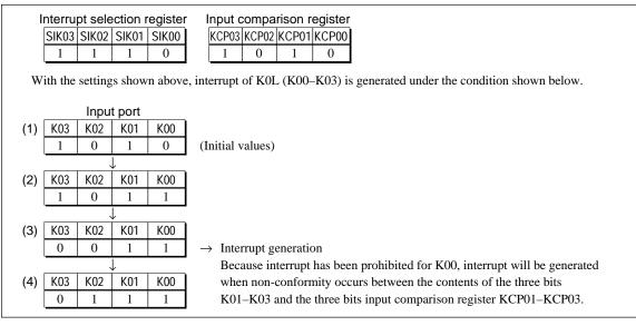
Fig. 5.4.3.2 Interrupt generation example in K0L (K00–K03)
