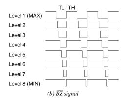
Fig. 5.12.3.1 Duty ratio of buzzer signal waveform
