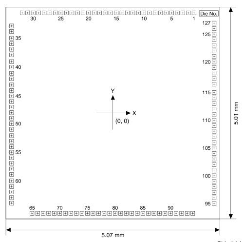
Chip thickness: 0.4 mm Pad opening: 95 μm
