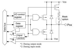
Fig. 5.6.1.1 Structure of I/O port
