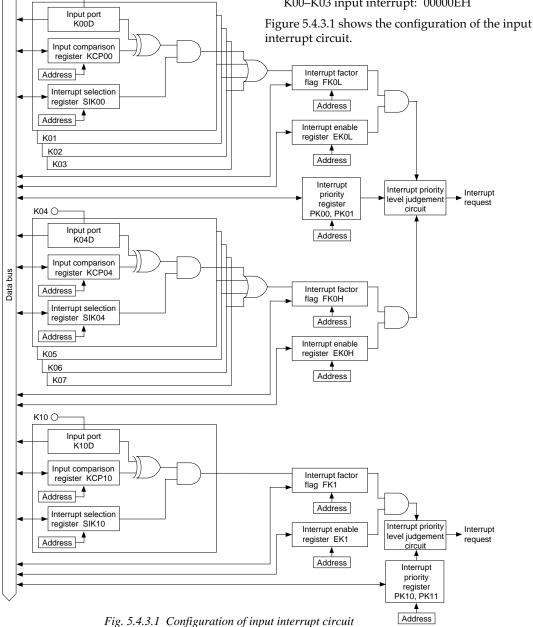
The interrupt selection registers SIK00–SIK03, SIK04–SIK07 and SIK10 and input comparison registers KCP00–KCP03, KCP04–KCP07 and KCP10 for each port are used to set the interrupt generation condition described above.
