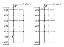
\* Vss level or high impedance when LCD is not driven.
