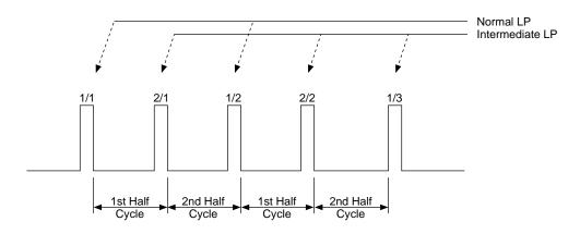
The segment output voltage during 1/2 H operation also follows the display data of 4.3 and the diagram showing the relationship between the LC AC signal FR and the segment output voltage. In the signal B/ A that indicates the number of the LP, the "A" in the figure indicates LP during a normal drive, and "B" differentiates between the normal LP and the intermediate LP (where B = 1 is normal and B = 2 is intermediate).
