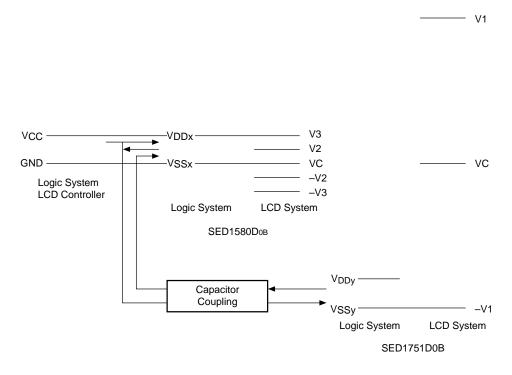
When the SED1580 and SED1751 are used to structure an extremely low-power module system, the power supplies for the SED1580 logic systems and LCD systems, and the power supplies for the LCD controller should have the voltage relationships shown in the figure above.
