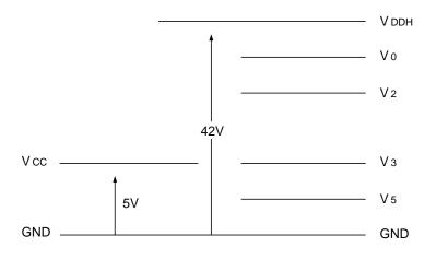
(Note 4) If the logic operation power goes into a floating state or if VCC drops to 2.6V or below while the LCD driving power is being applied, the LSI may be damaged. Therefore, keep from occurrence of the aforementioned status. Specifically, pay close attention to the power supply sequence at times of turning the system power on and off.
