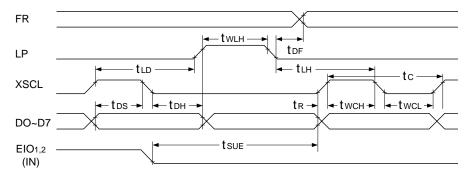
$V_{CC} = 5.0V \pm 10\%$ ,  $T_a = -30$  to  $85^{\circ}C$
