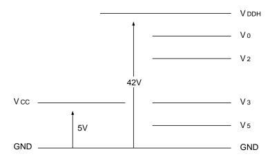
(Note 4) If the logic operation power goes into a floating state or if VCC drops to 2.6V or below while the LCD driving power is being applied, the LSI may be damaged. Therefore, keep from occurrence of the aforementioned status.
