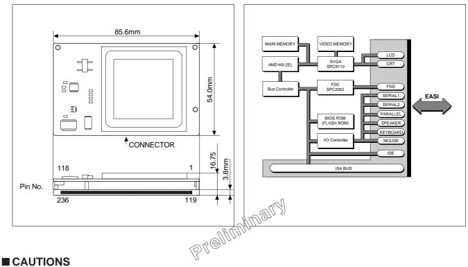
There is danger of burns because the surface of CARD-686 gets very hot. We ask for the safty measure not to touch the surface or setting up the cover. The prominent precaution about the temperature are requested.
