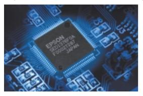
Using a guaranteed low-latency CPU architecture, SED1376 provides support for microprocessors without READY/WAIT# handshaking signals. The 32-bit internal data path provides high performance bandwidth into display memory, allowing for fast screen updates.
