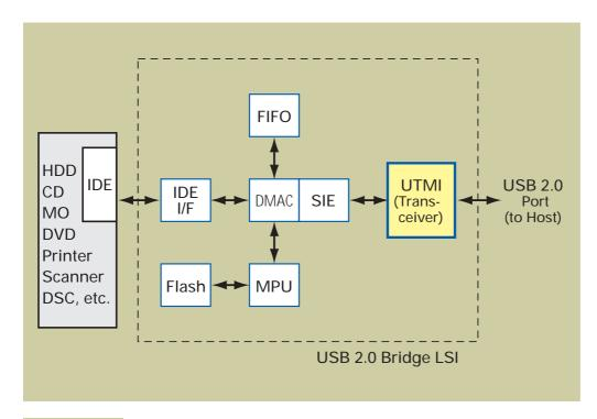
USB (Universal Serial Bus) is a standard for serial buses connecting PCs and peripherals. As an evolution of the USB 1.1 specification it has basically the same behaviour but a much higher bandwidth. USB 2.0 enables high speed data transfer of up to 480 Mbits/second. This feature opens the door to higher performance peripherals such as fast storage devices, next generation printers and scanners or even video-conferencing cameras.
