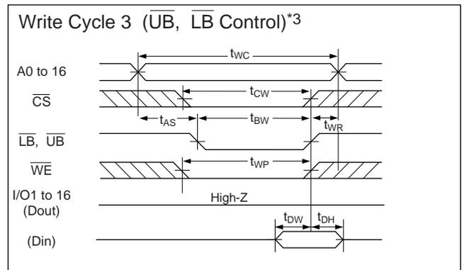
Note : \*1 During read cycle time,  $\overline{WE}$  is to be "High" level.
