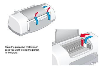
3. Attach the printer parts
