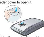
5 Open the film guide. Secure the film guide by pushing down the front end of the film guide gently until you hear a click.
