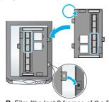
B. Film (the last 3 frames of the film strip). Reverse the position of the film holder and place it against the right edge of the scanner.
