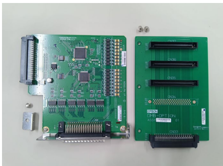
Optional board (as needed) / L-shaped bracket MAIN-OPTION board / 3 mounting screws
